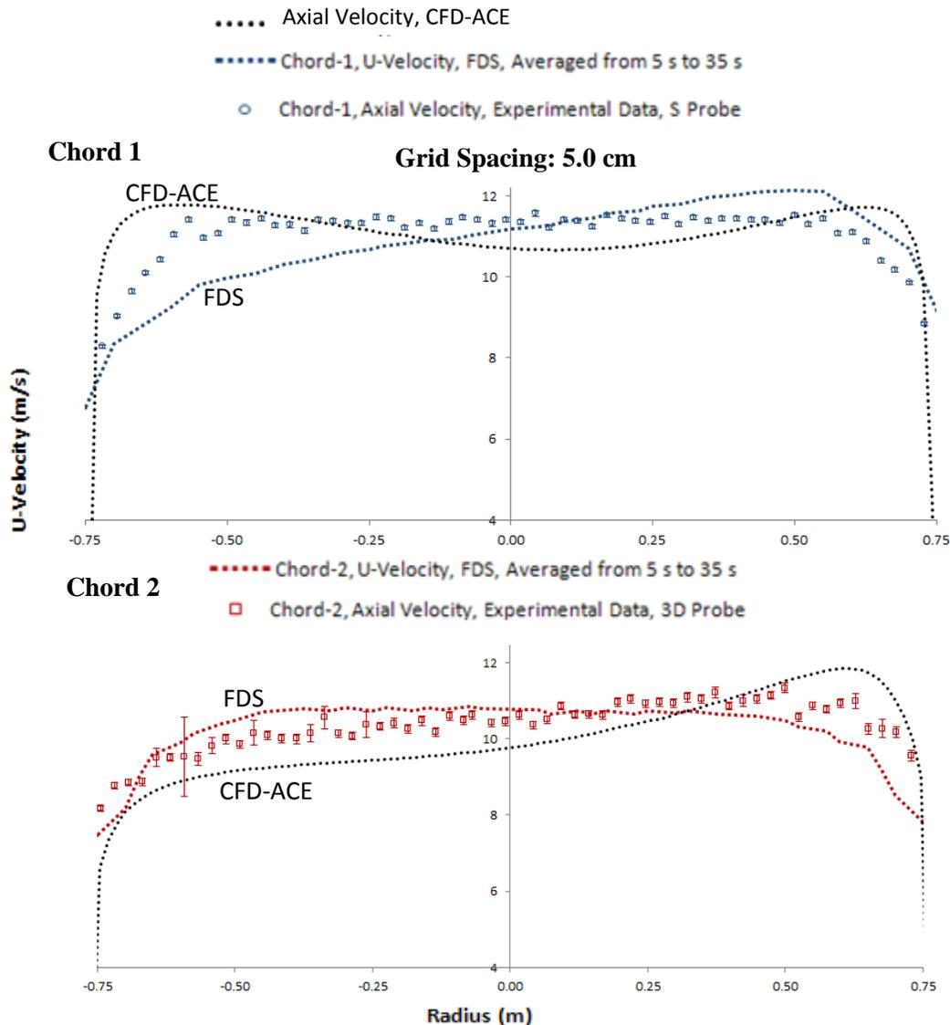
**Figure 13: Comparison of FDS simulation results, CFD-ACE data and experimental measurements for axial velocity plotted as a function of duct radius. Results are shown for Chord 1 (top sub-figure) and Chord 2 (bottom sub-figure).**
