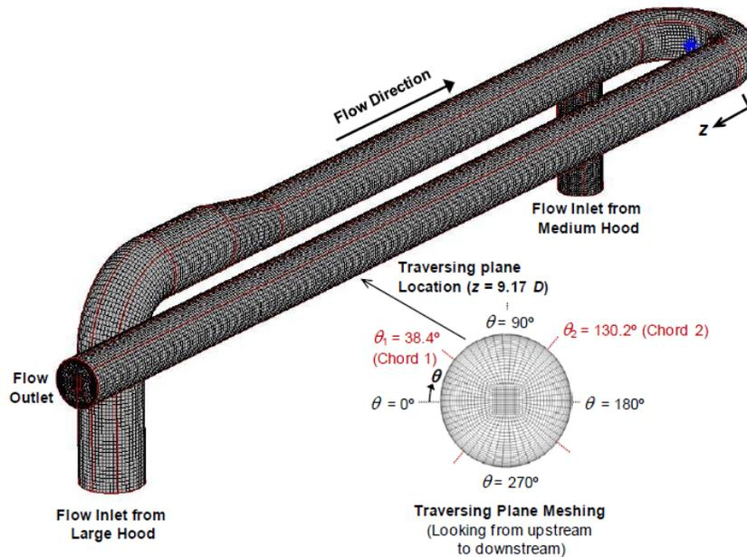
**Figure 4: Isometric view of the CFD-ACE model that was used for simulating the flow through the NFRL exhaust duct. Direction of flow is indicated as well as the chords on the measurement plane, from an upstream to downstream view [6].**
