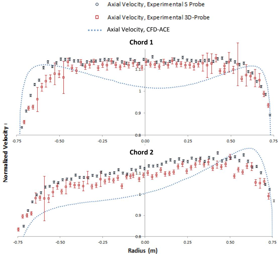
**Figure 3: Measured and CFD-ACE results for axial velocity profiles for Chord 1 (top) and Chord 2 (bottom), normalized by annubar velocity. Results are shown for cold flow with the large hood inlet, with experimental measurements from the S Probe and 3-D probe. Relative expanded uncertainty of the velocity inferred from the S-probe (1.0 %) and 3-D probe (4.1%).**
