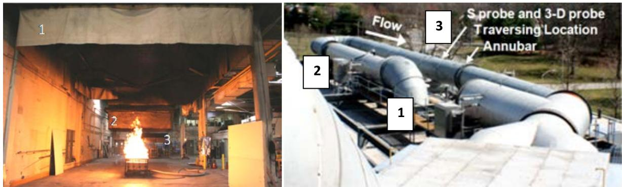
**Figure 1: Left: the natural gas burner below the large hood, labeled 1, Right: top view of the exhaust duct above the NFRL. The large hood inlet is labeled as 1, the medium hood inlet is labeled as 2, and the measurement plane is labeled as 3.**
