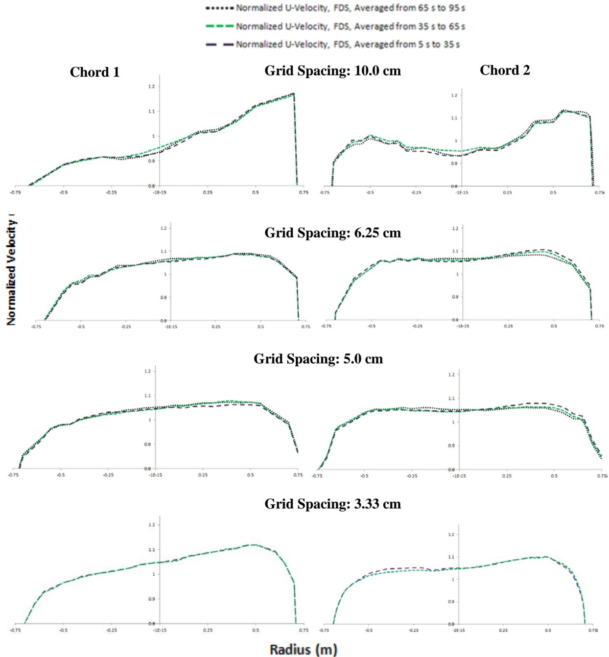
**Figure 12: Convergence studies of simulated FDS results. Results for Chord 1 are shown on the left, those for Chord 2 are shown on the right. The grid spacing used was 10.0 cm, 6.25 cm, 5.0 cm and 3.33 cm. The axial velocity is normalized by dividing by an area weighted velocity.**
