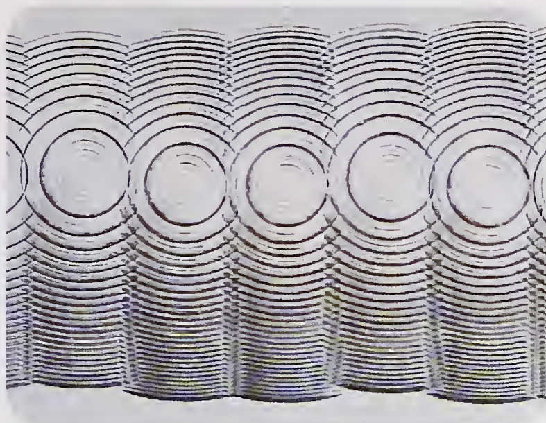
Photomicrograph of an array of multilevel diffractive lenses, fabricated with a 193 nanometer excimer laser.
