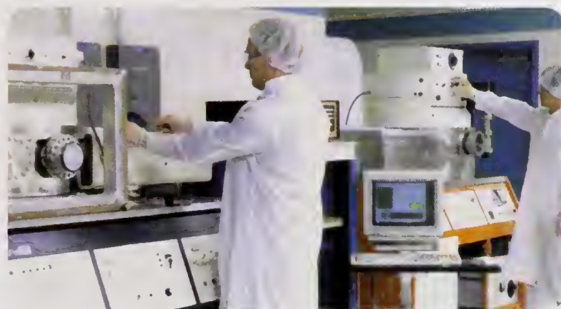
The clean room at Nonvolatile Electronics in which GMR sensors and other devices are fabricated.
