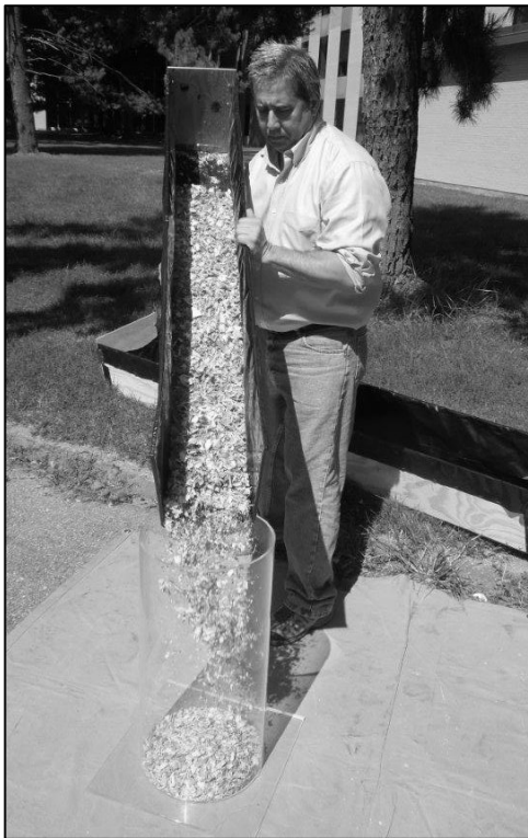
Figure 3-23. Filling a 44 L Test Measure.
