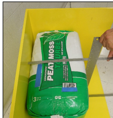
Figure 3-6. Width Measurement. The frame is rotated on its end to vertical so that the carpenter square does not compress the product.
