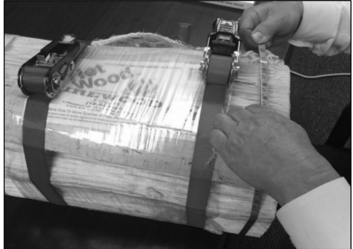
Figure 3-17. Strapping the Ends of a Bundle.
