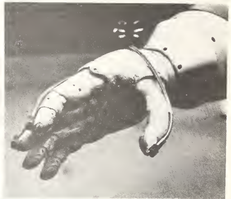
Figure 8. JPL/Ames Arm with Humanoid Hand Equipped with Three Miniaturized Proximity Sensors
