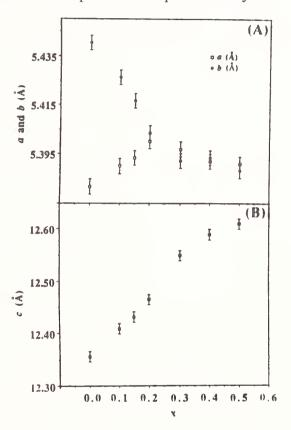
Figure 3. A) Change in the lattice parameters a and b as a function of  $Ca^{2+}$  content in  $Nd_{2-}$   $_xCa_xNiO_{4+}\delta$ , B) Change in the lattice parameter c as a function of  $Ca^{2+}$  content in  $Nd_{2-x}Ca_xNiO_{4+}\delta$ .
