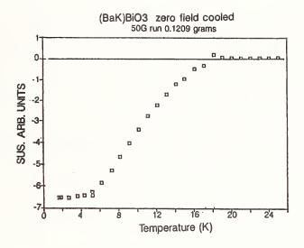
Figure 2 Susceptibility Plot for BKBO Polycrystalline Mass
