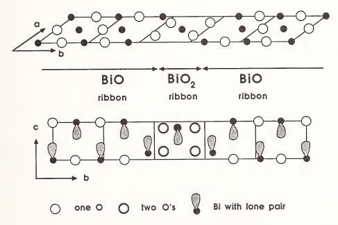
Figure 8. Schematic representation of the effect of the introduction of extra oxygen in the BiO layer. In the oxygen rich region the lone pairs point no longer to an oxygen of the adjacent BiO layer allowing a shorter BiO-BiO layer distance as is indicated in b).
