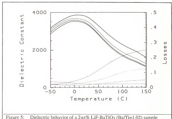
Dielectric behavior of a 2wt% LiF-BaTiO<sub>3</sub> (Ba/Ti=1.02) sample sintered at 900° for 2 h. Figure 5:
