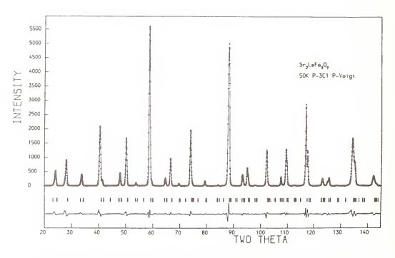
Figure 10: Neutron diffraction pattern of Sr<sub>2</sub>LaFe<sub>3</sub>O<sub>8.94</sub> at 50K
