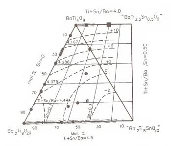
Fig. 6.  $T_f$  isopleths (approximate) for the system  $BaTi_4O_9$ - $Ba_2Ti_9O_{20}$  and  $SnO_2$ -containing solid solutions (1330-1350°C, $O_2$ ). Hatching depicts approximate limits of solid solubility after (1) and this work ( $\blacksquare$ , not single phase). Open circles are after (5).
