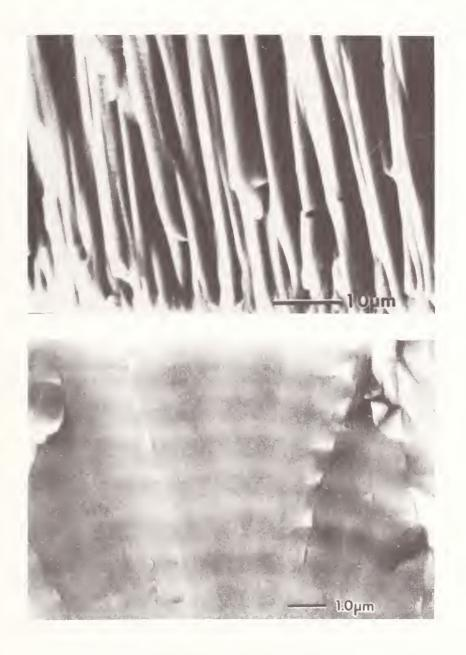
Figure 2. Scanning electron micrographs of modulated  $Tl_aPb_bO_c/Tl_dPb_eO_f$  films. Micrographs are low (top) and higher (bottom) magnifications of a cross-sectional view of a fractured film. Film was deposited by cycling electrode between 0.05 mA and 5 mA in a solution of 0.005 M  $TlNO_3$  and 0.1 M  $Pb(NO_3)_2$  in 5 M NaOH. Layer thicknesses are intentionally quite thick (~0.5  $\mu$ m) so that SEM imaging is possible.
