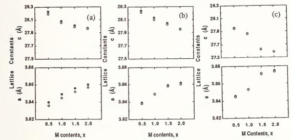
Fig. 4. Relationship between lattice constants and metallic ion content, x, for  $(Eu_{3/4}Ce_{1/4})_4(Eu_{1/3}Sr_{2/3})_4Cu_{6-xM_N}C_z$  with (a)M=Fe, (b)M=Co and (c)M=Al. Close circles are for as-sintered samples and open circles for annealed samples at high oxygen partial pressure of 200 atm.
