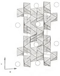
**Figure 5.** X-ray structure of  $SrTi_{11}O_{20}$ : (a) unit cell projected along the *b*-axis; (b) A-layer, and (c) B-layer, projected along the *a*-axis.
