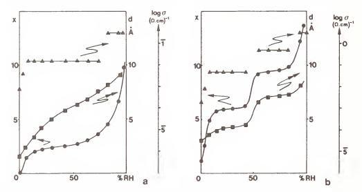
Fig. 4 - Adsorption isotherm of water, evolution of the water content x, of the interlayer distance d and of the conductivity, as a function of the relative humidity at  $20^{\circ}$ C for a)  $\mathrm{HSb(PO_4)_2.xH_2O}$  b)  $\mathrm{H_3Sb_3P_2O_{14}.xH_2O}$ .
