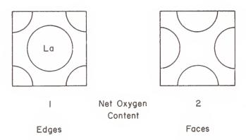
Fig. 5. (a) Cross-section through a NaCl-type layer in  $\text{La}_2\text{CuO}_4$  with oxide ions on the cell edges and lanthanum in the center. (b) The corresponding shifted layer of oxide ions in Nd $_2\text{CuO}_4$  that have moved to the faces without a central cation.
