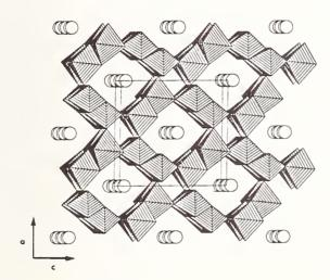
Figure 6. Polyhedral representation of the X-ray structure of La<sub>0.3</sub>Ti<sub>2</sub>O<sub>4</sub>.
