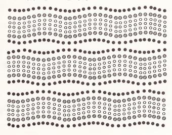
Figure 6. Schematic representation of the modulated structure of Bi<sub>2</sub>Sr<sub>2</sub>CaCu<sub>2</sub>O<sub>8+∂</sub>. Only the cations are shown (black=Bi, white=Cu, small shaded=Ca, large shaded=Sr).
