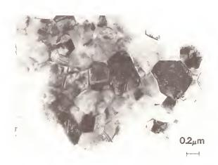
Figure 1. Transmission electron micrograph of Y-TZP (2.75 mol%  $\rm Y_2O_3,$  grain size = 0.35  $\mu m$  ).
