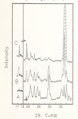
Fig. 18. XRD tracings for ceramics in Fig. 17 (A,B,C correspond to E' = 45, 55, 68, respectively). A =  $LT_2 + L_2T_9 + t$  trace ordered perovskite (P, shaded); B =  $LT_2 + L_2T_9 + P$ ; C =  $L_2T_9 + P$  (trace  $LT_2$ ).  $LT_2 = La_2Ti_2O_7$ ;  $L_2T_9 = La_4Ti_9O_{24}$ .
