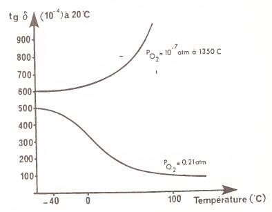
Figure 3: Influence of the oxygen partial pressure during the sintering of a Z5U material with general formula Ba<sub>1-x</sub> Ca<sub>x</sub> Ti<sub>1-y</sub> Zr<sub>y</sub> O<sub>3</sub> [3].
