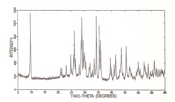
Figure 5. X-ray powder diffraction pattern of the reaction between molten  $Ba(NO_3)_2$  and Au foil at 650°C in one atmosphere of  $O_2$ . This pattern shows no  $BaO_{2-x}$ ,  $Ba(NO_3)_2$  or Au.
