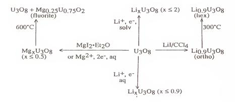
Fig 3: Insertion Reactions of  $\alpha$ -U<sub>3</sub>O<sub>8</sub>
