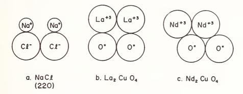
Figure 4. (a) Side view (220 plane) of the ideal NaCl structure with R = 0.414R . (b) Side view of NaCl-type part of the  $^{\rm C}$ La $_{\rm 2}$ CuO $_{\rm 4}$  structure with R = R . (c) The lateral shift of a pair of ions that gives the more effective space-filling of the Nd $_{\rm 2}$ CuO $_{\rm 4}$  structure.
