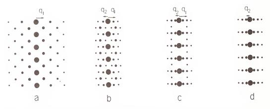
Figure 7. Schematic representation of [100] diffraction patterns of Bi2-xPbxSr2Ca1-yYyCu2O8+ $\partial$  with a) x=0,y=0.6, b) x=0.3,y=0.3, c) x=0.3,y=0.0, and d) x=0.6,y=0.0, showing a) the Bi-type of modulation, b) and c) the mixed Bi/Pb type of modulation, d) the Pb-type of modulation.
