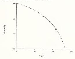
Fig. 2. Internal magnetic field vs. temperature for Y<sub>2</sub>SrFeCuO<sub>6.5</sub>
