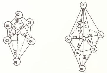
Fig 2: Oxygen Coordination About Uranium and Vanadium in UVO<sub>5</sub> [6]
