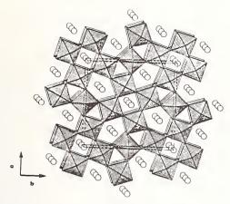
Figure 4. Polyhedral representation of the X-ray structure of Ba<sub>3</sub>Nb<sub>5</sub>O<sub>15</sub>.
