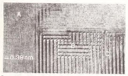
Figure 1. Micrograph of YBa<sub>2</sub>Cu<sub>3</sub>O<sub>7-∂</sub> showing [100] 90° rotation twin boundaries. For A, B, and C regions the c axis is out of the plane, vertical and horizontal respectively.
