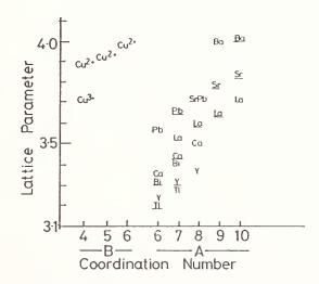
Figure 2. Lattice parameters expected for various AO and BO<sub>2</sub> layers with A and B cations in coordinations close to their AOCN (underlined).
