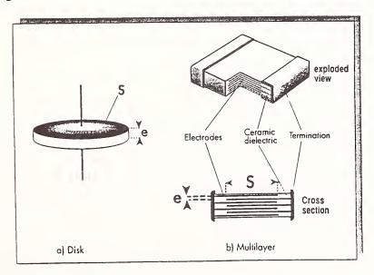
Figure 2: Ceramic Capacitors
