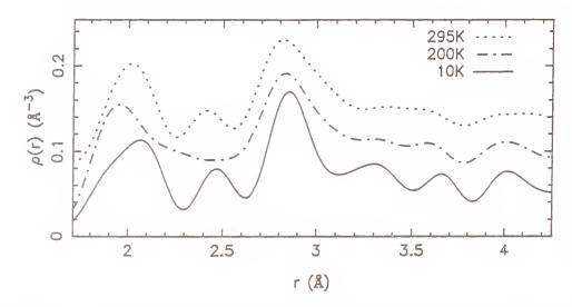
Figure 1. PMN Pair-distribution functions at 295K(dot), 200K(dot-dash) and 10K(solid).
