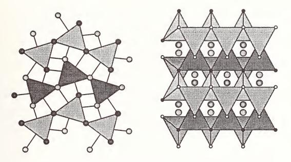
Fig. 1 SrD<sub>2</sub> showing Sr-centered Fig. 2 SrD<sub>2</sub> showing D(1)Sr<sub>4</sub> tricapped trigonal prisms. tetrahedra. Large balls D atoms are at 0 and 1/2. are D(2) atoms.
