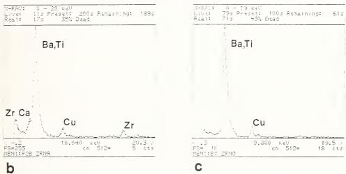
Fig. 7: TEM photomicrograph and corresponding EDS spectra of 90 mol % BaTiO<sub>3</sub>-8 mol % CaZrO<sub>2</sub> - 2 mol % TiO<sub>2</sub> ceramic, fired 2 hours at 1260°C.
