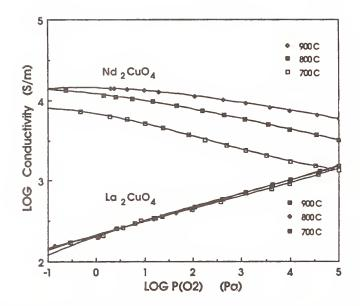
Figure 1. The equilibrium electrical conductivities of undoped La $_2^{\rm CuO}_4$  and Nd $_2^{\rm CuO}_4$  measured as a function of oxygen activity.
