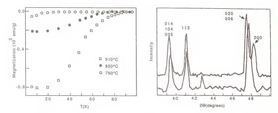
Figure 2. Magnetic susceptibility and X-ray diffraction data of samples of YBa<sub>2</sub>Cu<sub>3</sub>O<sub>7-3</sub> obtained by heating at various temperatures resulting in different densities of [100] 90° rotation twin boundaries. For high densities the superconducting fraction is very small and the material remains tetragonal (bottom line in X-ray plot).
