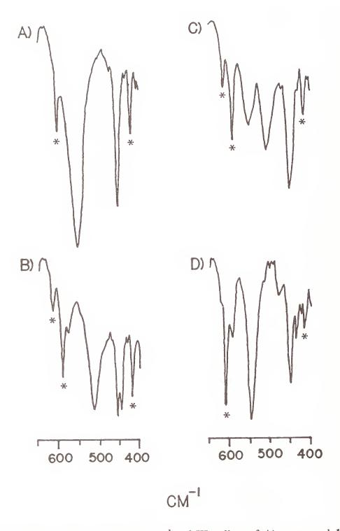
Figure 2. FTIR spectra (650-400 cm<sup>-1</sup>) of KI pellets of A) compound 1, B) compound 2, C) compound 3, and D) (C<sub>5</sub>H<sub>7</sub>O<sub>2</sub>)<sub>2</sub>Cu<sub>2</sub>(μ-OCH<sub>2</sub>C<sub>6</sub>H<sub>5</sub>)<sub>2</sub>.
