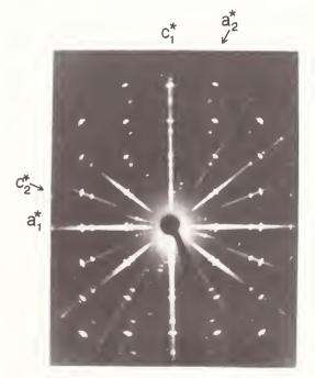
Figure 11d. hOl, unfiltered radiation, showing typical growth habit of multi (twinned?) crystals with the c\*-axis always inclined at the same angle  $(\sim76^{\circ})$ .
