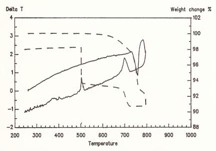
Figure 1b. DTA/TGA for  $BaO_2$ . Heating and cooling rates =5°C/min. Experiment performed in  $80~N_2/20~O_2$  heated to 800°C at 5°C/min, held for one hour, cooled to 500°C, held for 3 hours and cooled to 250°C.
