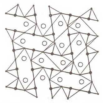
Fig. 2. Projection onto the (010) plane of the crystal structure of LaCuO<sub>25</sub>. The unit cell is drawn, see note to Fig. 1.
