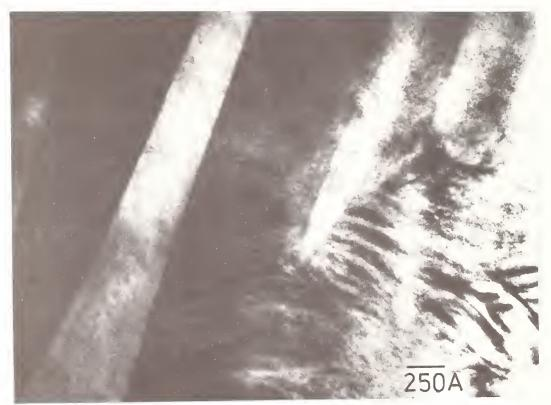
Fig 7 Ferroelastic and ferroelectric domains in rhombohedral PZT
