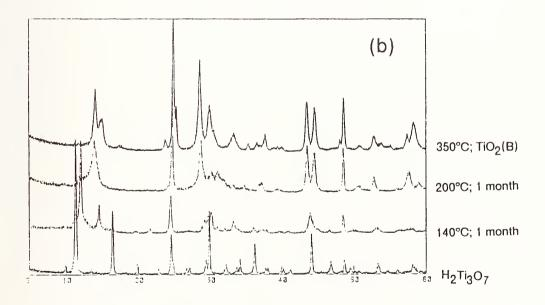
Figure 3. (a) Thermogravimetric analysis of layered titanates. (b) Powder X-ray diffraction of  ${\rm H_2Ti_3O_7}$  dehydration products.
