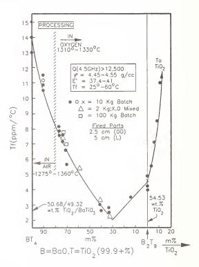
B<sub>2</sub>T<sub>9</sub> not unlike that proposed in (4). A Ba<sub>2</sub>Ti<sub>9</sub>O<sub>20</sub>-TiO<sub>2</sub>.
