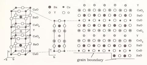
Figure 4. Representation of the atomic arrangement at a (001) grain boundary. The unit cell in perspective view and in [100] projection are given on the left. The grain boundary is either between the BaO and CuO planes or between the CuO<sub>2</sub> and BaO planes.
