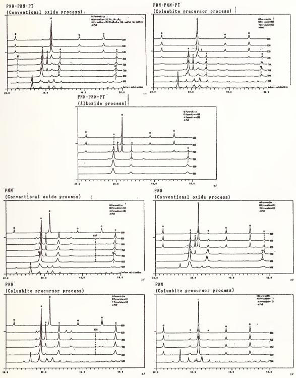
Figure 2 X-ray diffraction patterns of the calcined powder.
