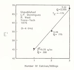
Fig. 17. "Processing" versus E' for "La<sub>2/3</sub>TiO<sub>3</sub>" composition.
