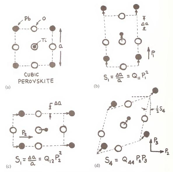
Fig. 1 Electrostriction in cubic pervoskite showing the physical origin of coefficients  $Q_{11},\,Q_{12},\,$  and  $Q_{44}.$
