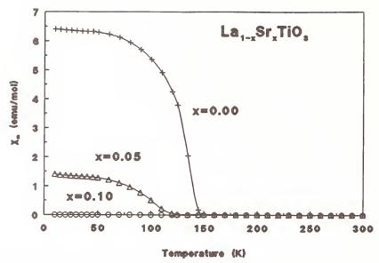
Figure 1. Magnetic Susceptibility data for  $La_{1-x}Sr_xTiO_3 x = 0, .05, .1$ .
