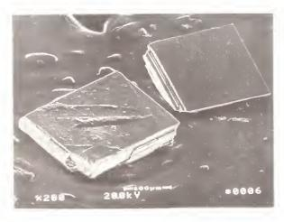
Figure 10. SEM photograph of crystals of  $BaO_{2-x}$  (courtesy J. Kelly).
