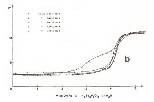
by the titrations Fig. 6 - Potentiometric titration curves for alkali alkali hydroxide solutions cations on a)  ${\rm HSb(PO}_4)_2.{\rm xH}_2{\rm O}$  b)  ${\rm H_3Sb_3P_2O_{14}.xH_2O}.$
