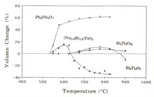
Figure 5. Volumetric expansion-shrinkage characteristics of Pb<sub>2</sub>Nb<sub>2</sub>O<sub>7</sub>, Bi<sub>2</sub>Ti<sub>2</sub>O<sub>7</sub> (pyrochlore), Na<sub>0.5</sub>Bi<sub>0.5</sub>TiO<sub>3</sub> (perovskite) and Bi<sub>4</sub>Ti<sub>3</sub>O<sub>12</sub> (larger structure).
