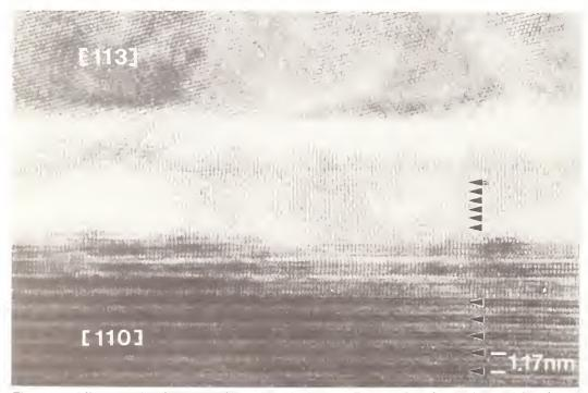
Figure 5. Micrograph of a grain boundary in La<sub>1.25</sub>Ba<sub>1.75</sub>Cu<sub>3</sub>O<sub>7-3</sub>, heated in nitrogen at  $950^{\circ}$ C for 24 hours, showing the presence of La<sub>2-x</sub>Ba<sub>x</sub>CuO<sub>4</sub> at the grain boundary. When this material is heated in oxygen atmosphere no second phase is formed.
