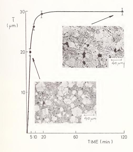
Fig. 1: Average intercept length vs. sintering time and corresponding microstructures for BaTiO<sub>3</sub> - TiO<sub>2</sub> excess ceramics, sintered at 1350°C
