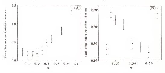
Figure 4. Room temperature electrical resistivity as a function of: A)  $Ca^{2+}$  content in  $Nd_{2-x}Ca_xNiO_{4+\delta}$ , and B)  $Ba^{2+}$  content in  $Nd_{2-x}Ba_xNiO_{4+\delta}$ .
