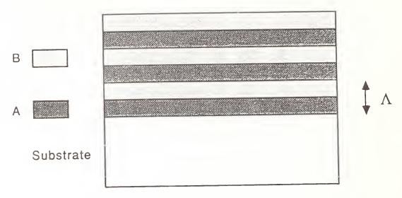
Figure 1. Idealized superlattice structure.
