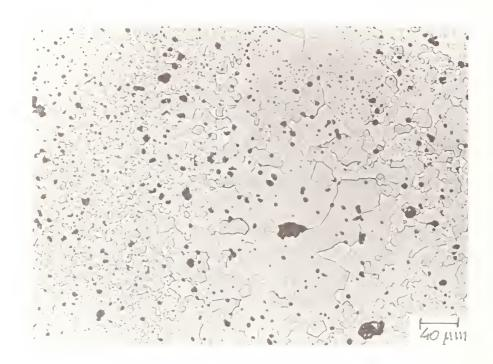
Fig. 3: Discontinuous grain growth in 95 w/o SrTiO<sub>3</sub> - 5 w/o BaTiO<sub>3</sub> ceramic sintered at 1450°C, 3 hours
