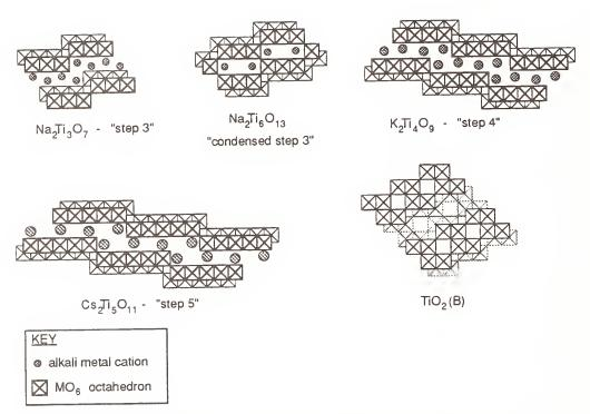
Figure 1. The structures of several alkali me al titanates and  ${\rm TiO}_2({\rm B})$
