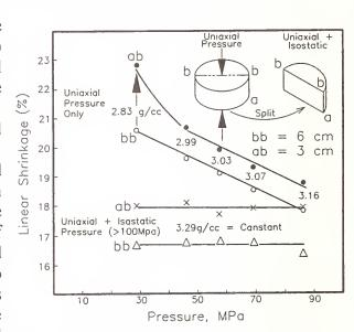
Fig. 11. Pressing methodology of  $\sim 1:1:4.5$ (Sm) powder (plus green densities) showing anisotropy in fired shrinkage.
