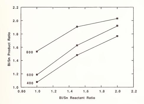
Figure 1. The dependence of the Bi/Sn ratio in  $Bi_2(Sn_{2-x}Bi_x)O_{7-x/2}$  on the ratio of the reactants and their concentrations used in the synthesis.
