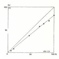
Fig. 8 - Disactivation curve (Propene Yield as a function of the IPA Conversion Yield) for  ${\rm H_3Sb_3P_2O_{14}.xH_2O}$ .
