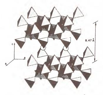
Fig. 1 - Perspective drawing of two  $(Sb(PO_4)_2)_n$  layers showing two potassium atoms in the interlayers space.
