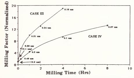
Figure 4. Milling factor (normalized) for reactively calcined PZT (Cases III (3.1  $\mu$ m) and IV (0.9  $\mu$ m)) as a function of milling (attrition) time.
