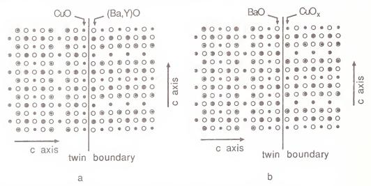
Figure 3. Atomic arrangement at [100] 90° rotation twin boundaries. From HREM images it cannot be determined which one of both structures occurs.
