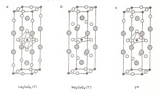
Fig. 1. The T, T' and T\* structures, Cu = solid circles, O = open circles and RE = shaded circles.
