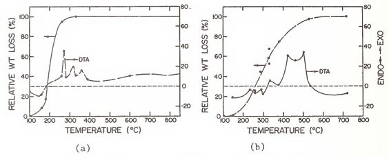
Fig 1. Relative Weight Loss (TGA) and Differential Thermal Analysis (DTA) of Polymeric Precursors for (a) LaMnO<sub>3</sub>. (b) BaTiO<sub>3</sub>.
