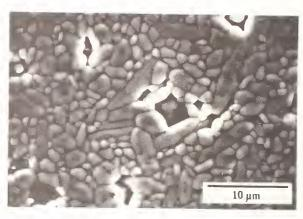
Fig. 10. Microstructure of ceramics in the vicinity of 1:1:4-1:1:5 (Sm<sub>2</sub>O<sub>3</sub>).
