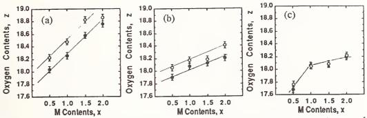
Fig. 3. Relationship between oxygen content, z. and metallic ion content, x, for  $(Eu_3/4Ce_1/4)_4(Eu_1/3Sr_2/3)_4Cu_{6-x}M_xO_z$  with (a)M-Fe, (b)M-Co and (c)M-Al. Close circles are for as-sintered samples and open circles for annealed samples at high oxygen partial pressure of 200 atm.
