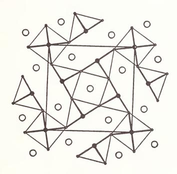
Fig. 1. Projection onto the (100) plane of the crystal structure of La<sub>5</sub>Cu<sub>5</sub>O<sub>13+y</sub>, with the unit cell indicated.
