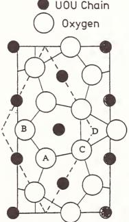
Fig 4: Sites for Insertion in  $\alpha$ -U<sub>3</sub>O<sub>8</sub> (z = 1/2)
