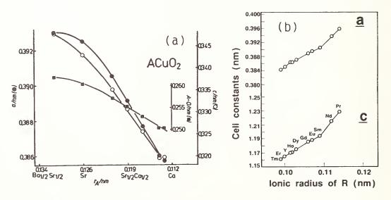
Fig. 8 Lattice constants and the A-O bondlength of  $ACuO_2$  (a) and the lattice constants of  $R_2CuO_4$  (T') (b).
