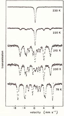
Figure 8: Mössbauer spectra of  $\rm Sr_2LaFe_3O_{8.94}$  as a function of temperature
