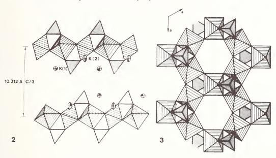
Fig. 2 -  ${\rm K_3Sb_3P_2O_{14}}$  : projection of the structure on (110).
