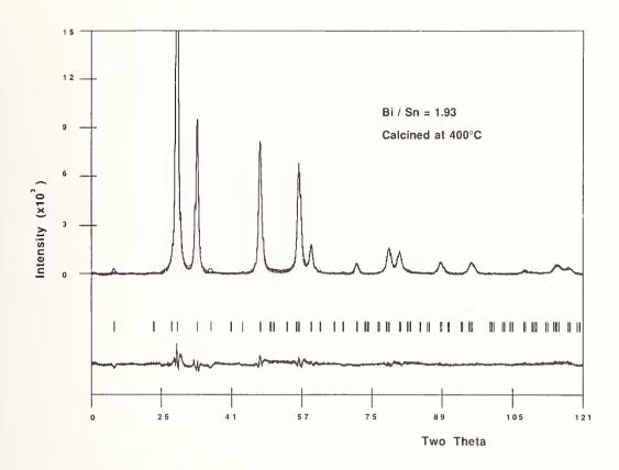
Figure 3. A room temperature powder X-ray diffraction pattern of a  $Bi_2(Sn_{2-x}Bi_x)O_{7-x/2}$  phase with Bi/Sn = 1.9. The observed and calculated data are shown together with a difference plot. The vertical lines mark the positions of the contributing Bragg reflections.
