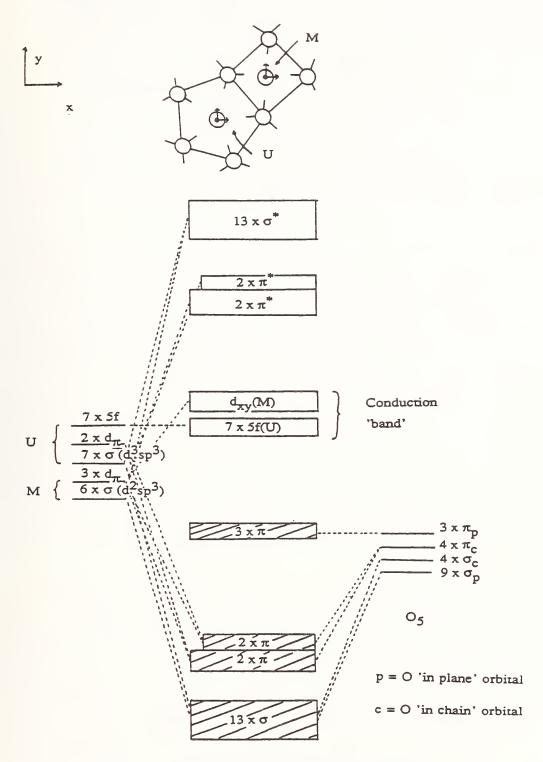
Fig 6: 1e<sup>-</sup> Energy-level Diagram for UMO<sub>5</sub>
