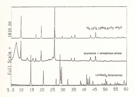
Figure 6. Powder X-ray diffraction of acid treated LiVMoO6.
