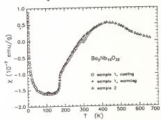
**Figure 3.** Magnetic susceptibility data for Ba<sub>2</sub>Nb<sub>15</sub>O<sub>32</sub> (uncorrected for Curie 'tail').
