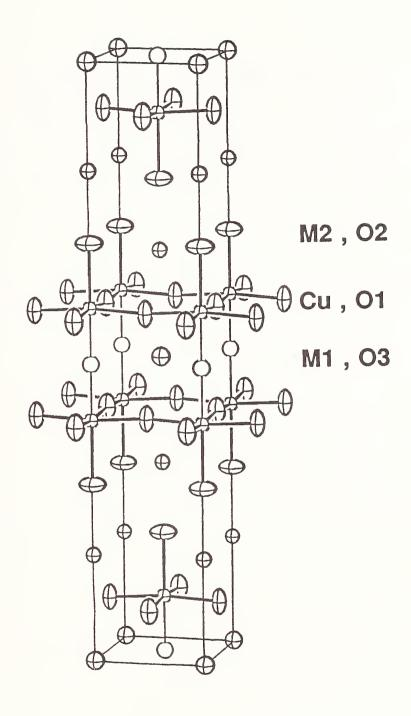
Figure 2. Structure of  $La_{1.85}Sr_{1.15}Cu_2O_{6.25}$ . Note that the O(3) site, which is completely vacant in the case of  $La_{1.9}Ca_{1.1}Cu_2O_6$ , is partially occupied in the present case.
