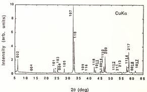
Fig. 2. X-ray diffraction pattern for  $(Eu_3/4Ce_1/4)_4(Eu_1/3Sr_2/3)_4Cu_4Co_20_z$  annealed at high oxygen partial pressure of 200 atm.
