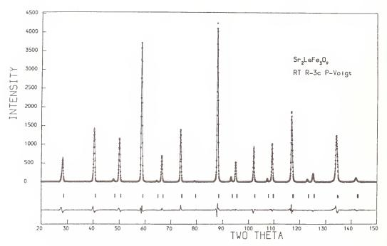
Figure 9: Neutron diffraction pattern of Sr<sub>2</sub>LaFe<sub>3</sub>O<sub>8.94</sub> at room temperature
