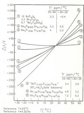
Fig. 8.  $\Delta f/f$  versus temperature ( $T_f = \Delta f/f\Delta T$ ) for ceramics based on  $Ba_2Ti_9O_{20}$  that contains various cation substitutions; 25-60, -30-25 in °C.
