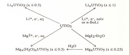
Fig 5: Insertion Reactions of UTiO5
