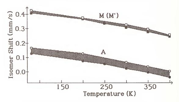
Figure 2. Mössbauer isomer shifts (relative to  $\alpha$ -Fe) for cobalt species A and M'(M) in YBa<sub>2</sub>Cu<sub>3</sub>( $^{57}$ Co)O<sub>6.27</sub> (open) and YBa<sub>2</sub>Cu<sub>3</sub>( $^{57}$ Co)O<sub>6.87</sub> (solid) as a function of temperature. Shaded areas are a guide to the magnitude of changes.
