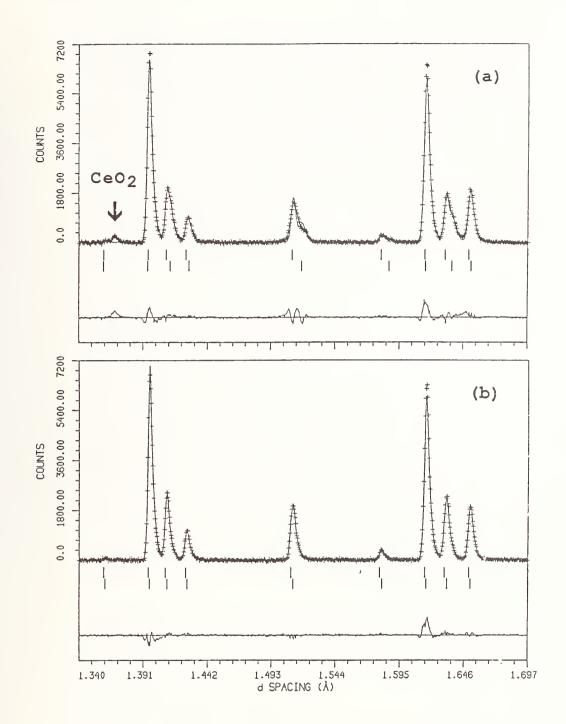
Fig. 2. Portion of the Rietveld refinement profiles for sample fired in air at  $1000^{\circ}$ C (a) and at  $1080^{\circ}$ C (b) followed by quenching.
