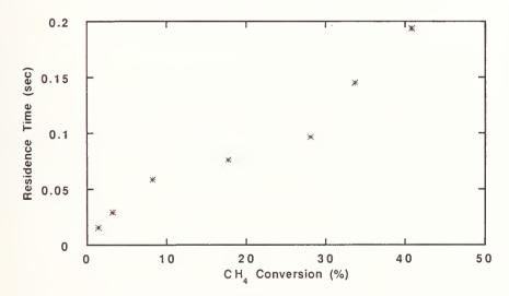
Figure 5. Product distribution at different conversions for a  $Bi_2(Sn_2-xBi_x)O_{7-x/2}$  catalyst with x = 0.71 at 850°C and CH<sub>4</sub>:  $O_2$ : Ar = 2:1:4 (top); residence time vs. conversion for the same catalyst (bottom).
