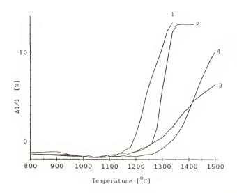
Fig. 5: Dilatometric curves for (1) BaTiO<sub>3</sub> - 2 mol % TiO<sub>2</sub> (2) BaTiO<sub>3</sub> - 2 mol % TiO<sub>2</sub> - 8 mol % CaZrO<sub>3</sub> (3) BaTiO<sub>3</sub> - 8 mol % CaZrO<sub>3</sub> (4) CaZrO<sub>3</sub>. Heating rates  $10^{\circ}$ C/min
