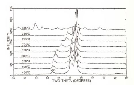
Figure 3. Portion of the x-ray powder diffraction patterns of quenched  $BaO_{2-x}$  heated at various temperatures, 450° - 735°C. Note change in the position of the (004) peak.
