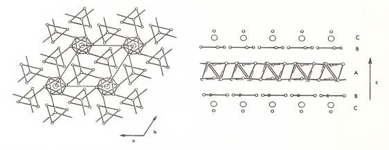
**Figure 1.** X-ray structure of  $Ba_2Nb_{15}O_{32}$ , projected along the c-axis (a), and perpendicular to it (b). Oxygen atoms omitted for clarity.
