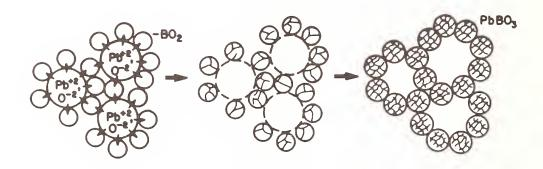
Figure 1. Schematic representation of the perovskite PbBO<sub>3</sub> formation and associated morphological changes.<sup>(3)</sup>
