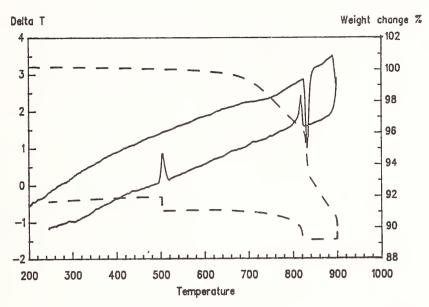
Figure 1a. DTA/TGA for  $BaO_2$ . Heating and cooling rates =5°C/min. Experiment performed in one atmosphere  $O_2$ , heated to 900°C, held for one hour, cooled to 500°C, held for one hour and cooled to 250°C.
