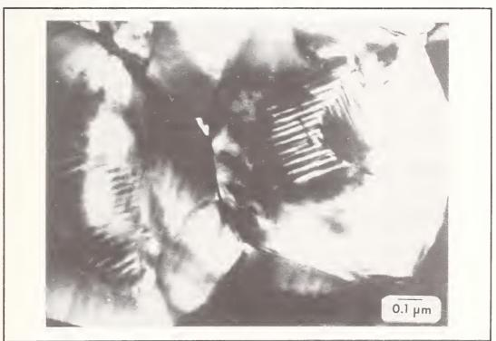
Figure 4: TEM micrograph of a 2wt% LiF-BaTiO<sub>3</sub> (Ba/Ti=1.02) sample sintered at 900°C.
