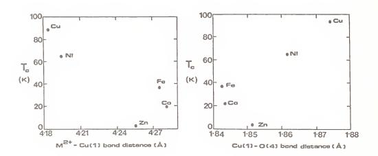
Fig. 2. Variation of T<sub>c</sub> with calculated bond distances for dopants on Cu(2). Observed values of T<sub>c</sub> from [2]
