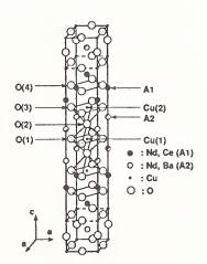
Fig. 1. Crystal structure of the 446 compound.
