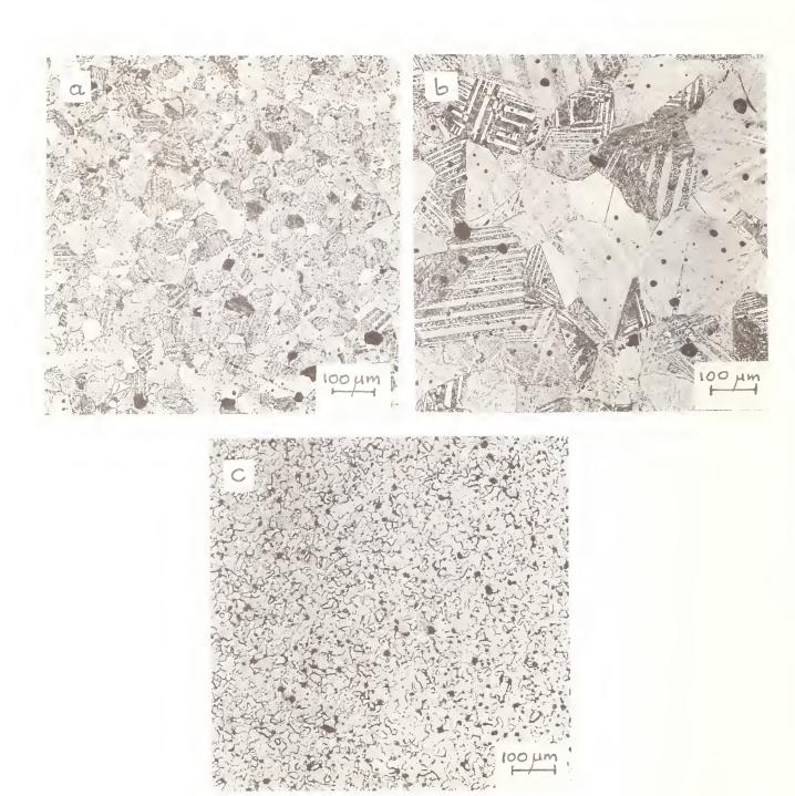
Fig. 2: Microstructures of BaTiO3 ceramics after heat treatment 24 hours at  $1350^{\circ}$ C (a) BaTiO3-2 mol % Ba6Ti<sub>17</sub>O<sub>40</sub>, (b) BaTiO<sub>3</sub> - 2 mol % Ba6Ti<sub>17</sub>O<sub>40</sub> - 8 mol % CaTiO<sub>3</sub>, (c) BaTiO<sub>3</sub> - 2 mol % Ba6Ti<sub>17</sub>O<sub>40</sub> - 8 mol % SrTiO<sub>3</sub>
