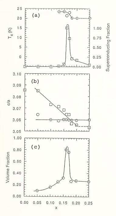
Fig. 1. Superconducting  $T_{\rm C}$  and volume fraction (a), lattice parameters ratio c/a (b) and volume phase fraction (c) as a function of starting cerium content for  ${\rm Nd}_{2-x}{\rm Ce}_x{\rm CuO}_4$ .
