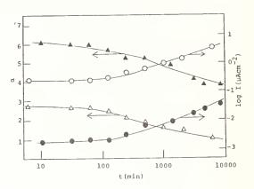
Fig. 2 Change in the non-ohmic exponent ( $\triangle$ ,  $\triangle$ ) and the current density under the bias (1V/cm) ( $\bigcirc$ ,  $\bigcirc$ ) with holding time at 25°C in dry air. Open and closed marks show the S-n and S-Co, respectively. The sample were prepared by quenching from 500°C into liq.N<sub>2</sub>
