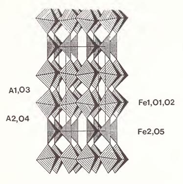
Figure 7: The crystal structure of  $Sr_2LaFe_3O_8$
