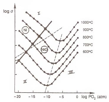
Figure 1: •—•— Equilibrium electrical conductivity versus oxygen pressure for undoped BaTiO<sub>3</sub> [1].
