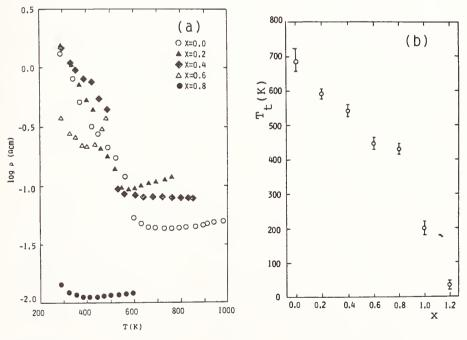
Fig. 7 Resistivity vs. T (a) and T  $_{\rm t}$  vs. x (b) data for  ${\rm La_{2-x}Sr_xNiO_4}.$
