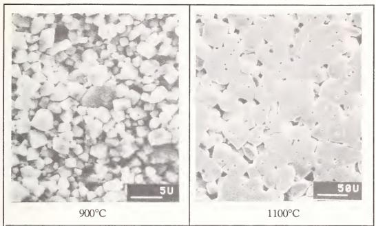
Figure 3: SEM micrographs of 2 wt% LiF-BaTiO<sub>3</sub> (Ba/Ti=1.02) sintered at 900°C and 1100°C for 2 hours.
