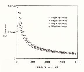
Figure 5. Magnetic susceptibility versus temperature of Nd<sub>1.8</sub>Ca<sub>.2</sub>NiO<sub>4.12</sub>, Nd<sub>1.7</sub>Ba<sub>.3</sub>NiO<sub>4.03</sub>, Nd<sub>1.4</sub>Ca<sub>.6</sub>NiO<sub>3.98</sub>, and Nd<sub>1.6</sub>Ba<sub>.4</sub>NiO<sub>3.99</sub>.
