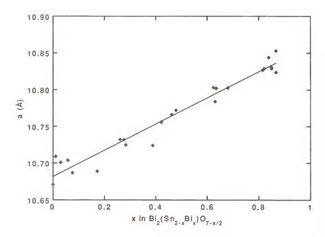
Figure 2. Lattice Parameter vs. Composition for Bi<sub>2</sub>(Sn<sub>2-x</sub>Bi<sub>x</sub>)O<sub>7-x/2</sub>.
