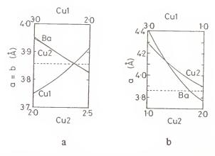
Figure 7. Modelled in-plane lattice spacings for the different layers of  $Ba_2YCu_3O_x$  assuming different distributions of the charge. a) for x = 7
