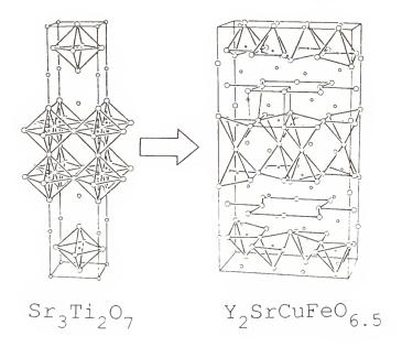
Fig. 1. The evolution of the Y<sub>2</sub>SrCuFeO<sub>6.5</sub> from the parent compound. Large circles are O, smaller circles are Y, and the smallest are Fe/Cu. The defect fluorite unit is outlined around one Y.
