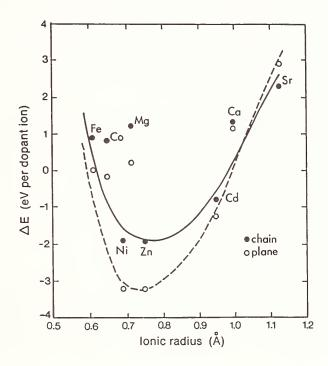
Fig. 1. Calculated solution energies versus divalent dopant radius
