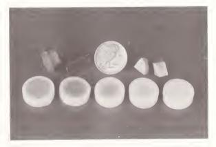
Fig. 3. Cored Ba<sub>2</sub>Ti<sub>9</sub>O<sub>20</sub> ceramics (1330°C, air). Slow cooled (bottom); air quenched (top); compositions from left to right correspond to materials in Fig. 2, left to right.
