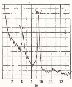
Figure 9. Low angle portion of x-ray powder diffraction pattern of reaction between a thin film of molten  $\text{Ba}(\text{NO}_3)_2$  and the outer wall of a Au tube, showing two phases "Hex"- "Ba $_6\text{Au}_3\text{O}_9$ " (9.75°  $_2\theta$ ) and "Tet" - "BaAuO $_{2.5}$ " (8.1°  $_2\theta$ ).
