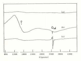
Fig. 4 ESR spectra for S-Co (a)spectrum for the sample evacuated at 600°C for 10 h. No signal was observed in this spectrum. (b)spectrum for the sample annealed at 500°C for 1 h in 130Pa of oxygen pressure and (c)spectrum for the sample exposed in 130Pa of oxygen pressure at 25°C after evacuation.
