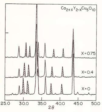
Figure 1. X-ray patterns for  $Ca_{2\pm x}Y_{2\pm x}Cu_5O_{10}$  with x=0, 0.4, 0.75. Shaded peaks due to incommensurate superstructures.
