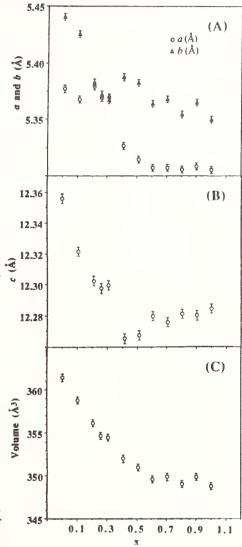
Figure 2. A) Change in the lattice parameters a and b as a function of  $Ca^{2+}$  content in  $Nd_{2-x}Ca_xNiO_{4+\delta}$ , B) Change in the lattice parameter c as a function of  $Ca^{2+}$  content in  $Nd_{2-x}Ca_xNiO_{4+\delta}$ , C) Change in the unit cell volume as a function of  $Ca^{2+}$  content in  $Nd_{2-x}Ca_xNiO_{4+\delta}$ .
