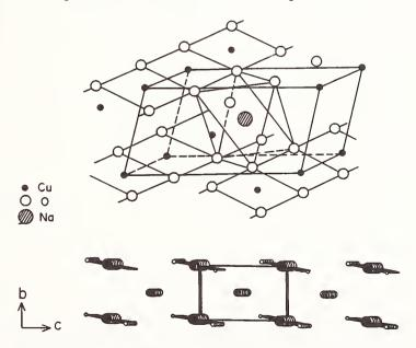
Figure 2. Schematic of NaCuO<sub>2</sub> structure. Edge-shared Cu square planes form 1-D chains along a axis. These are linked by larger cations located in channels.
