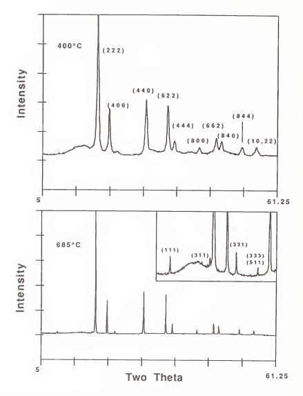
Figure 4. Comparison of the X-ray diffraction patterns for  $Bi_2(Sn_2-xBi_x)O_{7-x/2}$  with Bi/Sn = 1.06 at 430 and 685°C.
