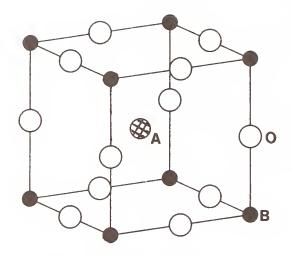
Figure 1: The perovskite structure
