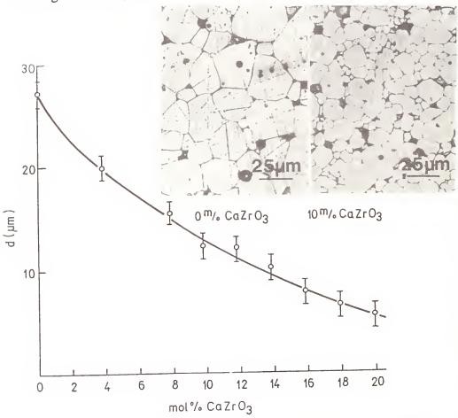
Fig. 6: Average grain size vs. composition in BaTiO3 - 2 mol % TiO2-CaZrO3 ceramics sintered 1 hour at  $1360^{\circ}$ C
