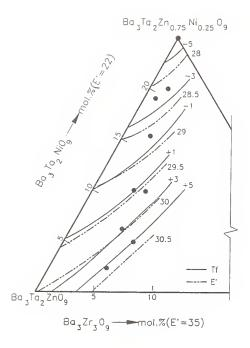
Fig. 16. T<sub>f</sub> and E' isopleths (approximate) for ordered perovskite ceramics in the system Ba<sub>3</sub>Ta<sub>2</sub>ZnO<sub>9</sub>-Ba<sub>3</sub>Ta<sub>2</sub>NiO<sub>9</sub>-Ba<sub>3</sub>Zr<sub>3</sub>O<sub>9</sub>. Ten Kg batches were made; fired densities are >7.70 g/cc.
