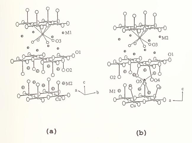
Figure 1. (a) Idealized tetragonal T\* structure, showing alternating T' (top half) and T (bottom half) layers. (b) The distorted T\* structure of  $La_{1.25}Dy_{0.75}CuO_{3.75}F_{0.5}$ , showing incorporation of the interstitial defect, O(5). Favorable coordination of O(5) to four M(1) and four displaced anion, O(4), sites occurs. Note that only half of the true unit cell (which is rotated by 45° around the c-axis, relative to (a)) is shown, for ease of comparison of the two structures.
