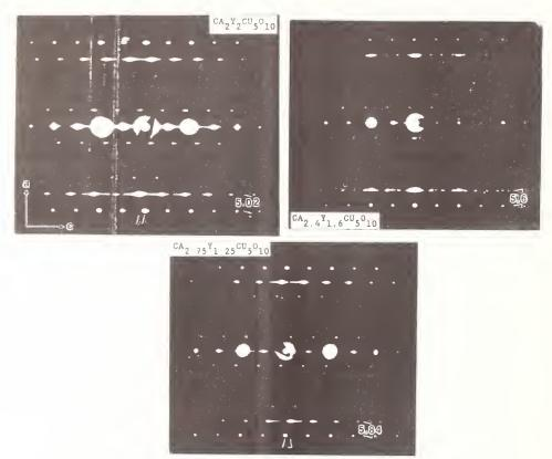
Figure 3. [010] diffraction patterns for a series of samples in the  $Ca_{2\pm x}Y_{2\pm x}Cu_5O_{10}$  system.
