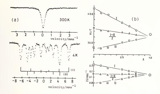
Fig. 1 Mossbauer spectra of CaFeO $_3$  (a) and IS and Hi of Ca $_{1-x}$ Sr $_x$ FeO $_3$  at 4K (b).
