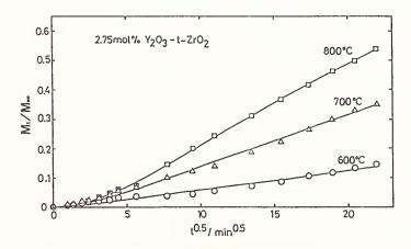
Figure 2. Typical results of diffusional annealing of Y-TZP (2.75 mol%  $\rm Y_2O_3$  , grain size = 0.35  $\mu m$  ).
