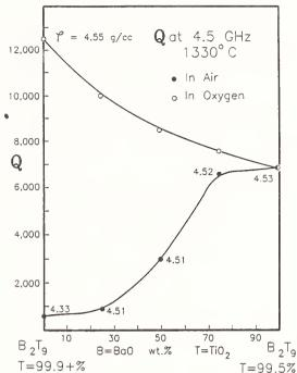
Fig. 1. Q of BaTi<sub>4</sub>O<sub>9</sub> ceramics versus TiO<sub>2</sub> raw material content. Temperature in °C.
