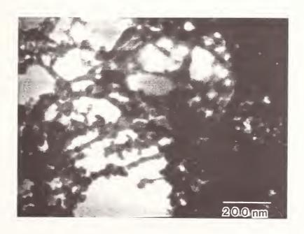
Figure 3. TEM micrograph of Y, Ba, and Cu hydroxycarbonates as coprecipitated in the chemical flow reactor.
