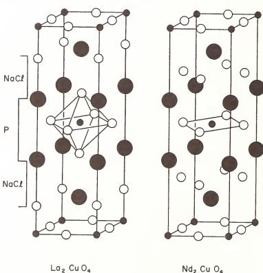
Figure 2. The crystal structures of La<sub>2</sub>CuO<sub>4</sub> and Nd<sub>2</sub>CuO<sub>4</sub>. Small solid circles are Cu; large solid circles are rare earth cations; open circles are oxygens. The alternate NaCl and perovskite (P) layers are indicated for La<sub>2</sub>CuO<sub>4</sub>.
