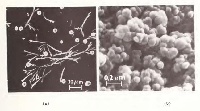
Figure 2. SEM micrographs of hydroxycarbonates conventionally coprecipitated at low-and high-ionic concentrations
