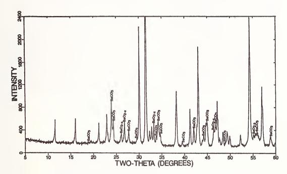
Figure 4. X-ray diffraction powder pattern of the reaction product obtained by heating a 40g batch of  $BaO_2$  in air on Au foil at  $700^{\circ}C$  - 20 min.
