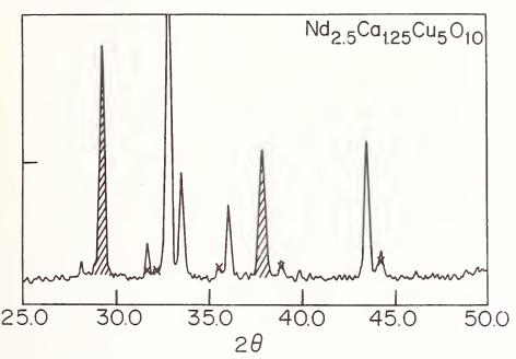
Figure 4. X-ray pattern of  $Nd_{2.5}Ca_{1.25}Cu_5O_{10}$ . Commensurate superlattice, peaks shaded, with a = 4asub, b=b, c=c.
