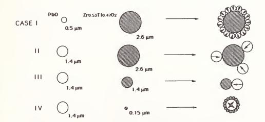
Figure 2. Component powder size schemes for the formation of perovskite PZT.
