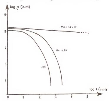
Figure 6: Resistivity of BaTiO3 based Z5U material as a function of various doping during life test (1.7V/µm and 280°C) [3].
