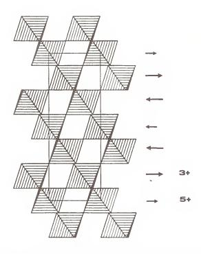
Figure 11: The magnetic structure of Sr<sub>2</sub>LaFe<sub>3</sub>O<sub>8.94</sub>
