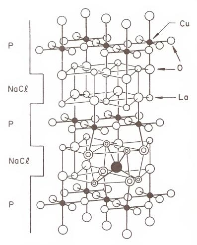
Figure 3. La<sub>2</sub>NiO<sub>4</sub> showing the interstitial oxygen (large solid circle) and the distorted cube of nearest neighbors (double circles).
