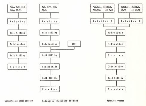
Figure 1 Processing flowchart for powder preparation.
