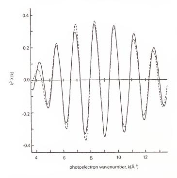
Figure 6: The Fourier-filtered EXAFS of the second coordination shell in 'rhombohedral'  $SrCoO_{2.5}$
