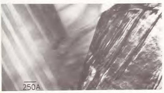
Fig 6 Edge-on (left) and inclined (right) ferroelectric domains in tetragonal PZT
