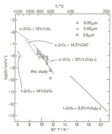
Figure 3. The diffusion coefficients in Y-TZP. Also shown are tracer diffusion in t-ZrO $_2$  doped with 14% CeO $_2$  [12], c-ZrO $_2$  doped with 12% Y $_2$ O $_3$  [10] and c-ZrO $_2$  doped with 14.2% CaO [9] and diffusivity calculated from electrical conductivity of Y-TZP (3.3 mol% Y $_2$ O $_3$ ) [14] and c-ZrO $_2$  doped with 12% Y $_2$ O $_3$  [13].
