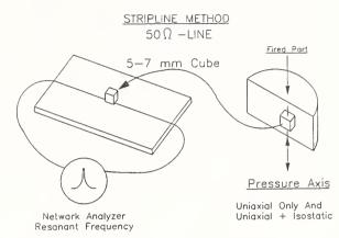
Fig. 12. T<sub>f</sub> of fired ceramics versus methodology of pressing (Fig. 11) and extraction of oriented test parts for electrical measurement.
