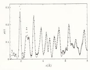
Figure 1. PDFs for Ca.85Sr.15CuO<sub>2</sub> from data taken at 10K (crosses) and best-fit model (line).
