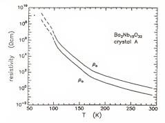
Figure 2. Single crystal resistivity data for Ba<sub>2</sub>Nb<sub>15</sub>O<sub>32</sub>.
