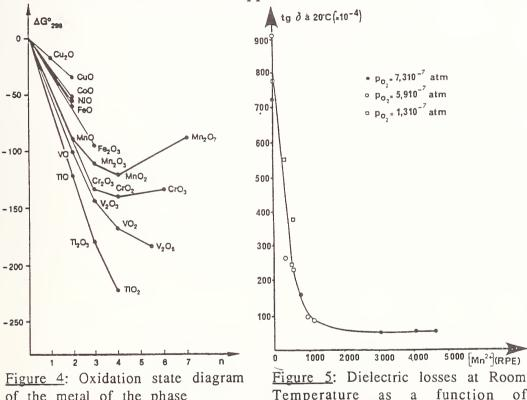
Figure 4: Oxidation state diagram of the metal of the phase transition series [4] (etablished with reference to the free enthalpy  $\Delta G^{0}280$  of formation of the oxides [7],[8]).
