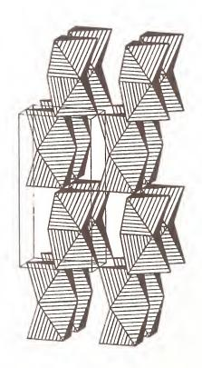
Figure 2: The crystal structure of  $SrMnO_3$
