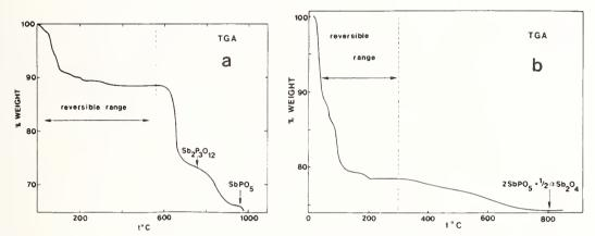
Fig. 5 - Weight loss versus temperature for a)  $HSb(PO_4)_2.xH_2O$  b)  $H_3Sb_3P_2O_{14}.xH_2O$ .
