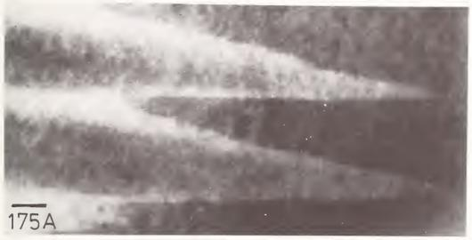
Fig 2b Lenticular 180° ferroelectric domains in BNN
