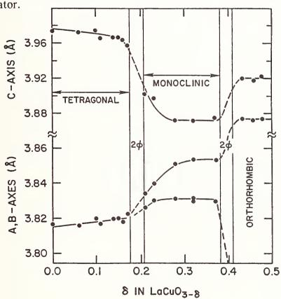
Fig. 3. The variation of the perovskite subcell parameters with oxygen content in LaCuO<sub>3- $\delta$ </sub>. The subcell *a*-axis of the orthorhombic phase (3.70 Å) is not shown for clarity,  $2\phi = \text{approx}$ . two phase region.
