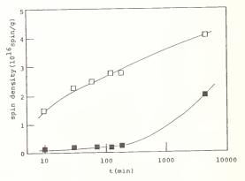
Fig. 3 Change in the spin density resulting from  $O_2^-$  and  $O_2^-$  for  $S_2^-$  n( $\bigcirc$ ) and  $S_2^-$  Co( $\bigcirc$ ).
