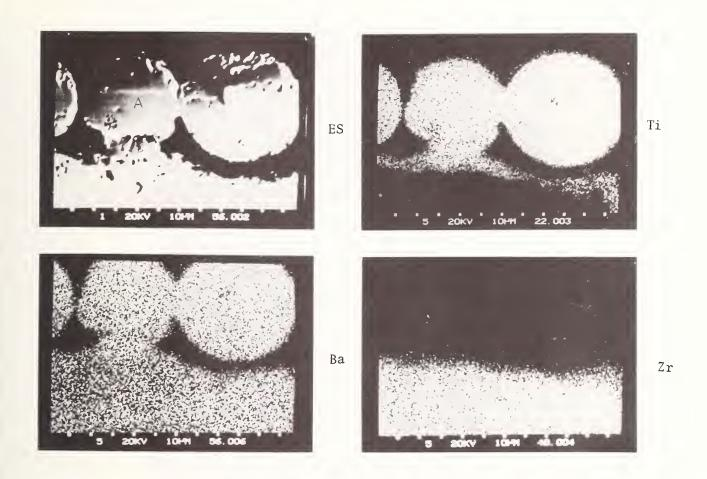
Fig. 4: Microprobe analysis of BaTiO<sub>3</sub> spheres sintered to BaZrO<sub>3</sub> plate at 1400°C, 3 hours. ES electron image, Ti, Ba, Zr X-ray image
