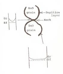
Fig.1 Cross Section of a connecting neck in a porous ZnO and its energy band.
