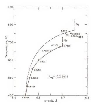
Figure 2. X-ray diffraction results of quenched  $BaO_{2-x}$  in air and " $O_2$ ". Temperature vs  $\underline{c}$ -axis derived from (004) peak.
