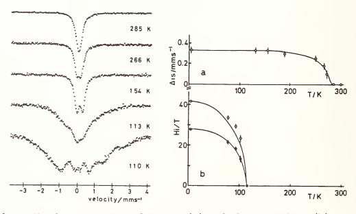
Fig. 4 Mossbauer spectra of CaFeO<sub>3</sub> (a) and the parameters (b).
