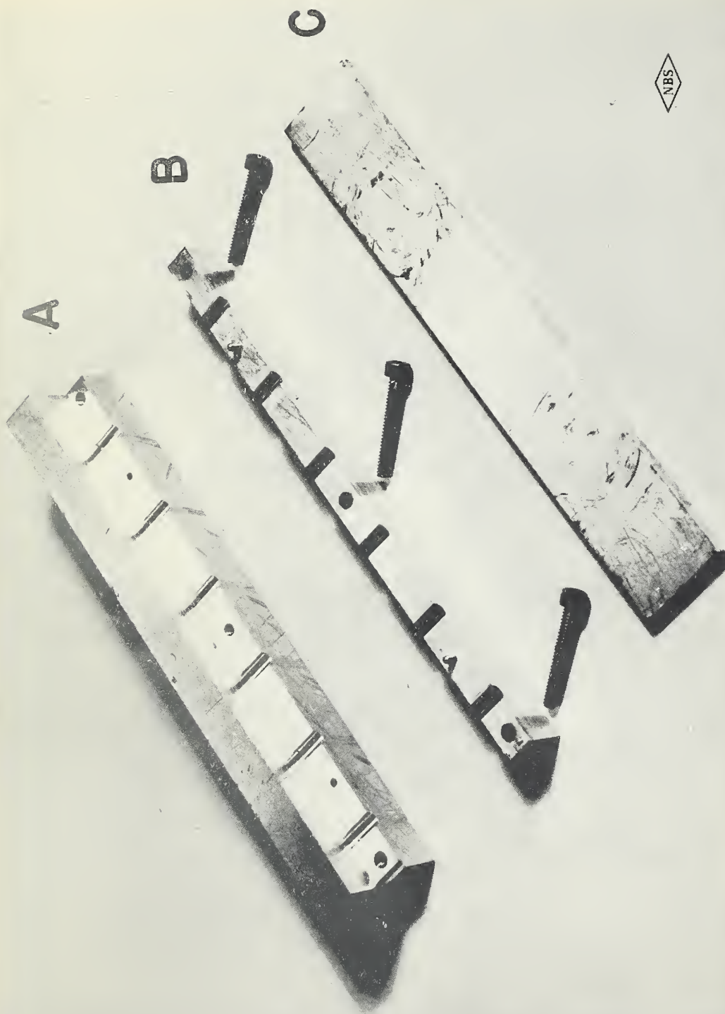
Fig. 1. Apparatus used to mold specimens for stress-strain measurements. Part B fits into part "A" and is fastened by screws. The cavities are then packed, steel plate is applied, and pressure is obtained by screw-clamps.
