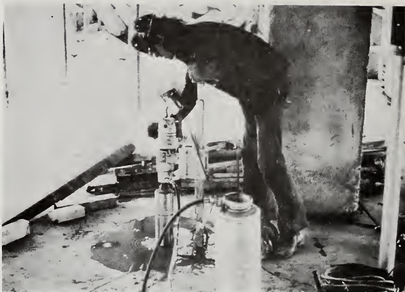
TAKING A CORE SAMPLE FROM A CONCRETE SLAB
