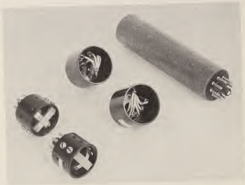
FIGURE 1.17. Typical plug-in units.
