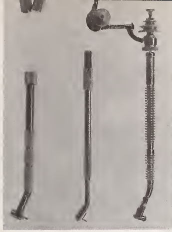
The high-speed turbine drill now so familiar in every dentist's office is a direct descendant of the first hydraulic-turbine handpiece developed at NBS in 1953, shown here with a conventional handpiece.
