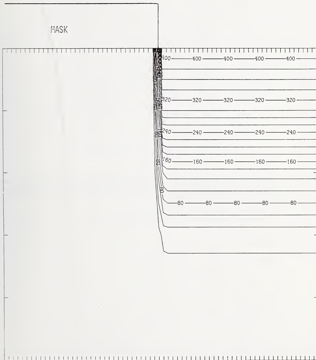
Figure Ge25-4 Two-dimensional distribution of Frenkel pairs created by 25 keV germanium implanted past a mask edge. The length increment (distance between tick marks) is 0.01 \mu\text{m} and the scale factor is 1.
