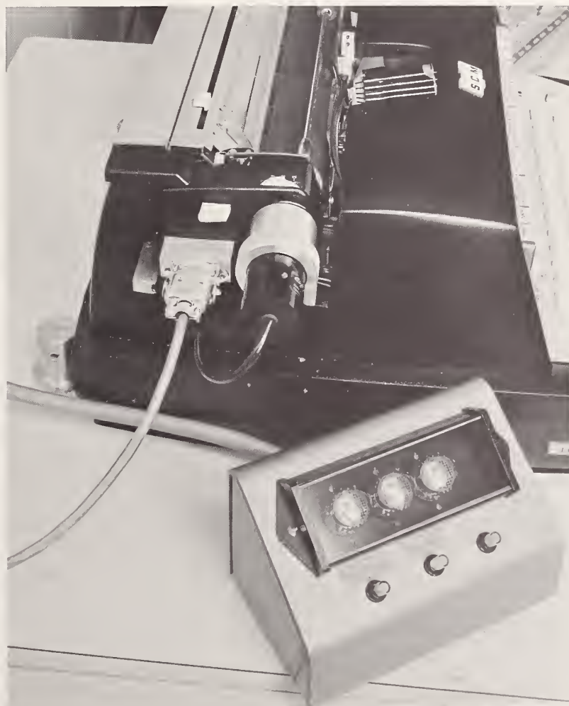
FIGURE 2. A close-up of the Taxywriter showing the platen rotation sensor and the Typit code display unit.
