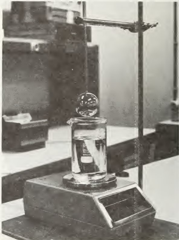
Figure 4. Gammaball fixed to rod
