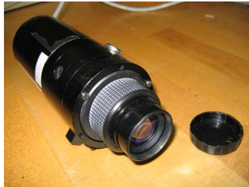
Fig. 7. Picture of the NV radiometer transfer standard with the PVS-7 input optics and the attached amplifier unit.
