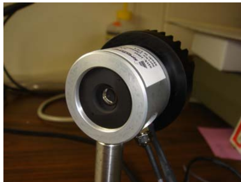
Fig. 1. A temperature-controlled pyroelectric transfer-standard radiometer head.
