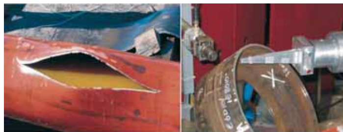
FIGURE 1: Left: Circumferential rupture in the hydrotest, and Right: measurement geometry for the corresponding hoop direction.
