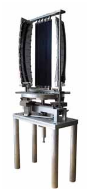
The Double Crystal Analyzer Linkage (DXAL) is one of 20 being installed in the Multi-Axis Crystal Spectrometer (MACS). Visible are two curved panels holding pyrolytic graphite crystals and collimating blades between them. The design features a single mechanical linkage that allows rotation of each crystal panel by 2\theta and each blade by \theta while maintaining parallel entering and exiting beam paths.
