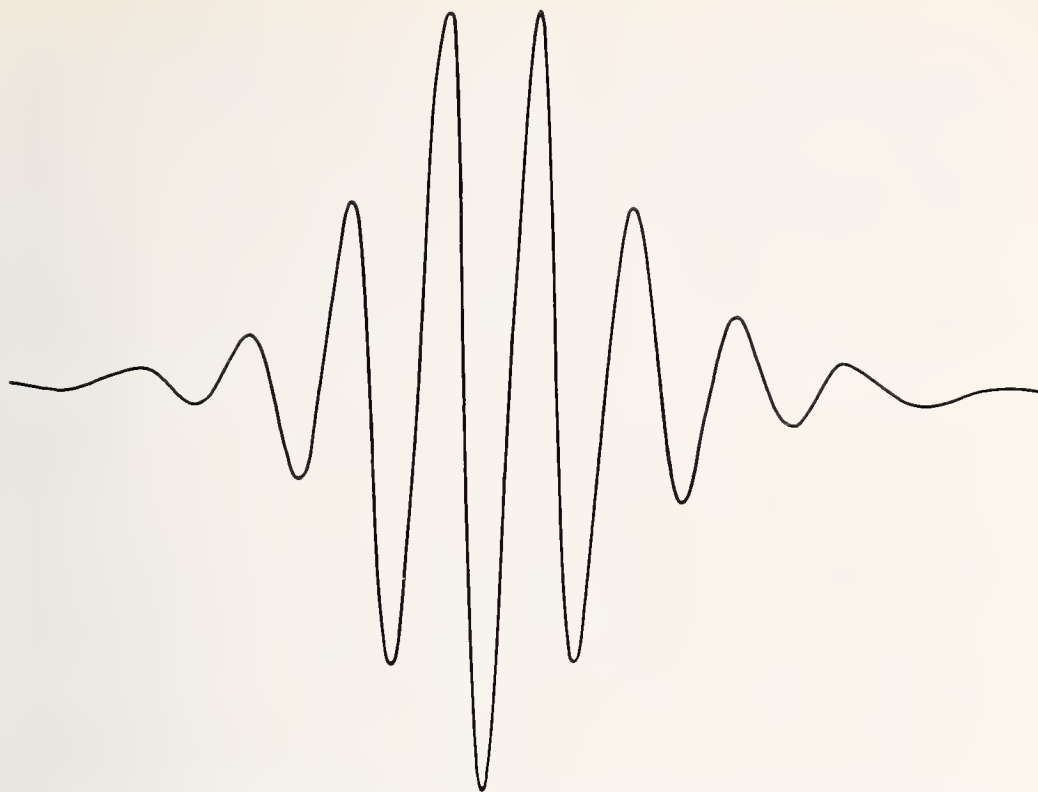
Figure 4. Image observed on the oscilloscope screen. When one observes a packet of several fringes, approximately centered on the oscilloscope screen, the adjustment is reached (the length of the packet corresponds to a carriage displacement of less than 1\ \mu\text{m} ).
