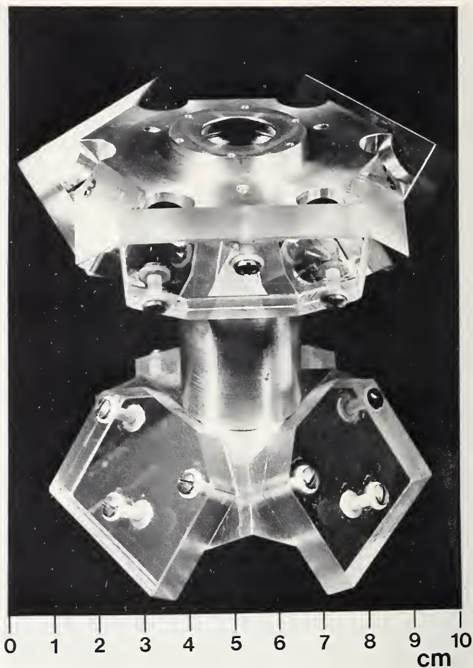
Figure 4. Projectile (mass 430 g) for the measurement of g by the two-station method. There are shown the six plane mirrors forming two corner reflectors back-to-back at the apex, the openings for the passage of light, and the central bore for the passage of the elastic cord of the catapult.
