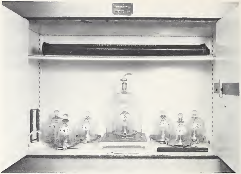
Vault for the metric prototypes. above : the International Metre of 1889 in its metal case; below : the International Kilogram \mathfrak{K} , under its three glass domes, and its six check standards. On the lower level are seen two thermometers, one of which is a maximum-minimum, and on the left a hair hygrometer.
