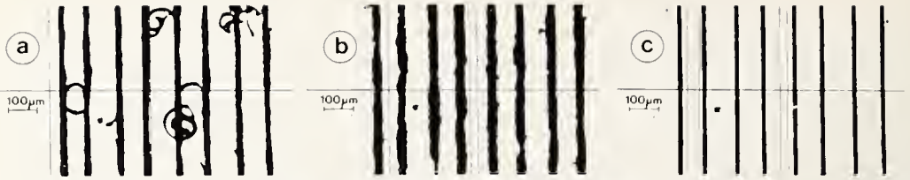
Figure 2. Appearance of lines engraved on a platinum-iridium prototype: (a) before trimming; (b) during trimming; (c) after trimming. The narrow lines are the wires of the reticle of the micrometer ocular.
