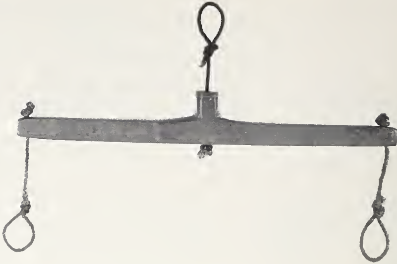
Balance of around 5000 B.C., found in a prehistoric tomb in Nagada in Egypt; length of beam \approx 8.5 cm (Courtesy Petrie Museum, University College London).
