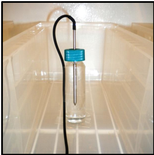
Fig. 5. Digital data logger probe correctly installed inside a glycol-filled bottle.
