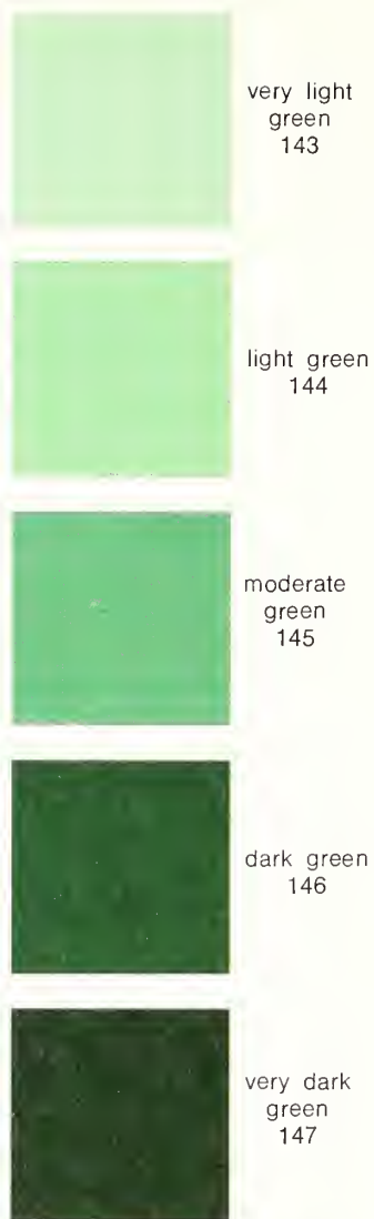
FIGURE 4. A photograph illustrating the value or lightness scale with five Centroid Colors: very light green, light green, moderate green, dark green and very dark green.
