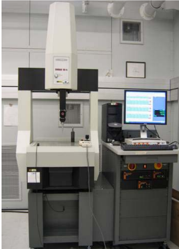
Figure 27. NIST Coordinate measuring machine.
