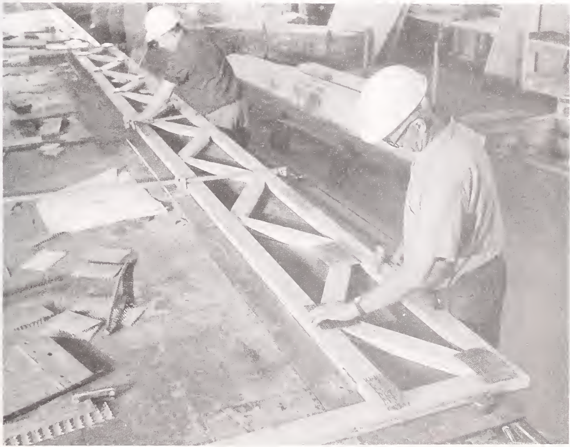
Figure 2. Unitized truss frames are fabricated in a plant to insure maximum quality control and material efficiency.
