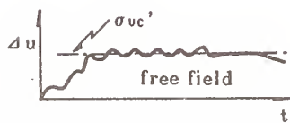
Fig.12 Estimation of the Effective Overburden Pressure from Pore Pressure Record
