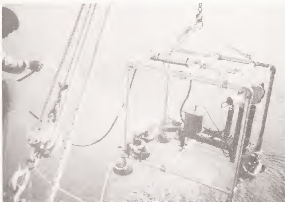
Figure 2. The Coastal Structure Acoustic Raster Scanner is raised from its underwater surveying position.
