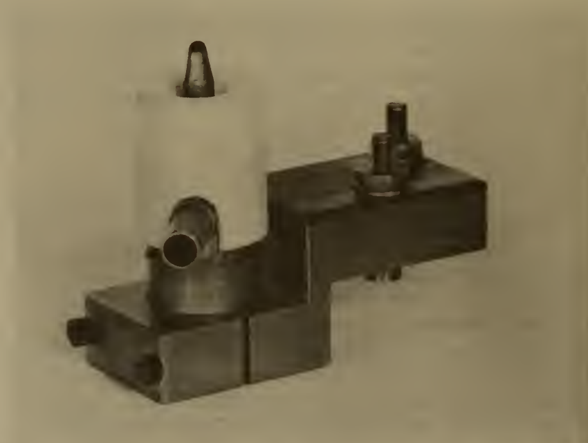
Figure 2. Device used for atmosphere control in inert-gas spark excitation.
