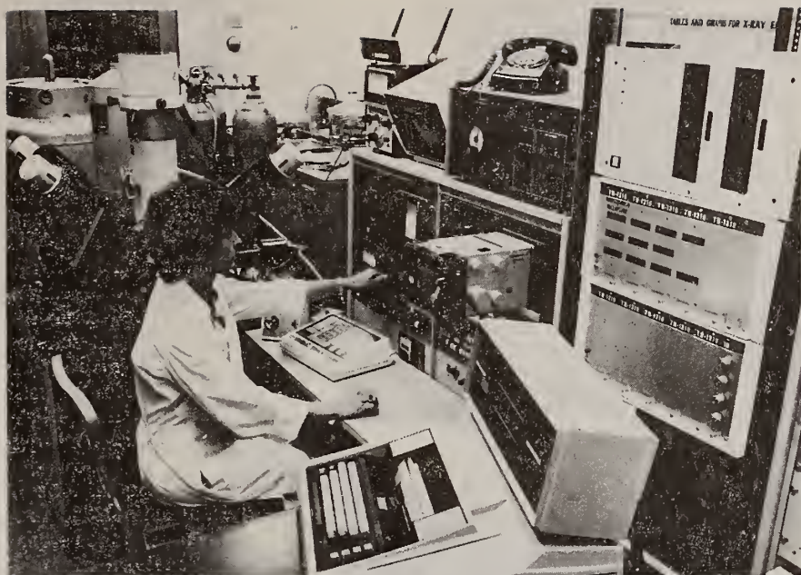
Ryna B. Marinenko operates an electron microprobe used for quantitative evaluation of microhomogeneity of SRMs such as SRM 470, mineral glasses
