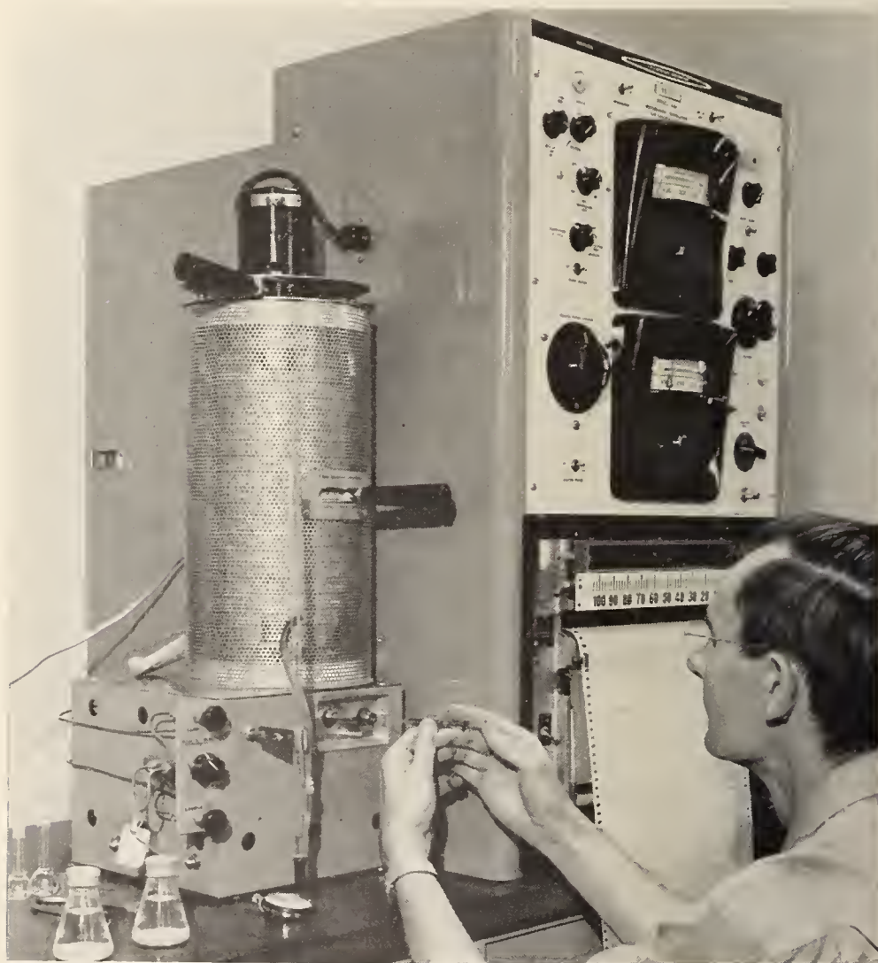
FIGURE 1.—A small amount of an alcohol-water extract from grain is injected into a gas chromatograph. The relative amounts of water and alcohol are recorded as separate peaks on a chart.
