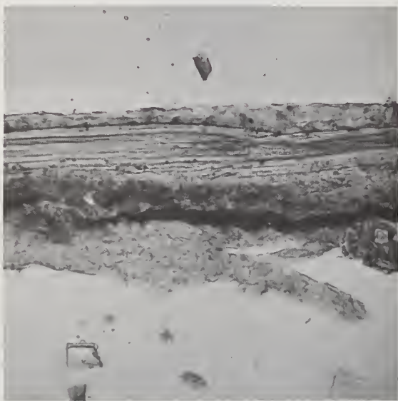
Figure 7. Microtome cut of Papyrus EBERS, shows between the two layers of papyrus the layer of starch adhesive – 120X.
