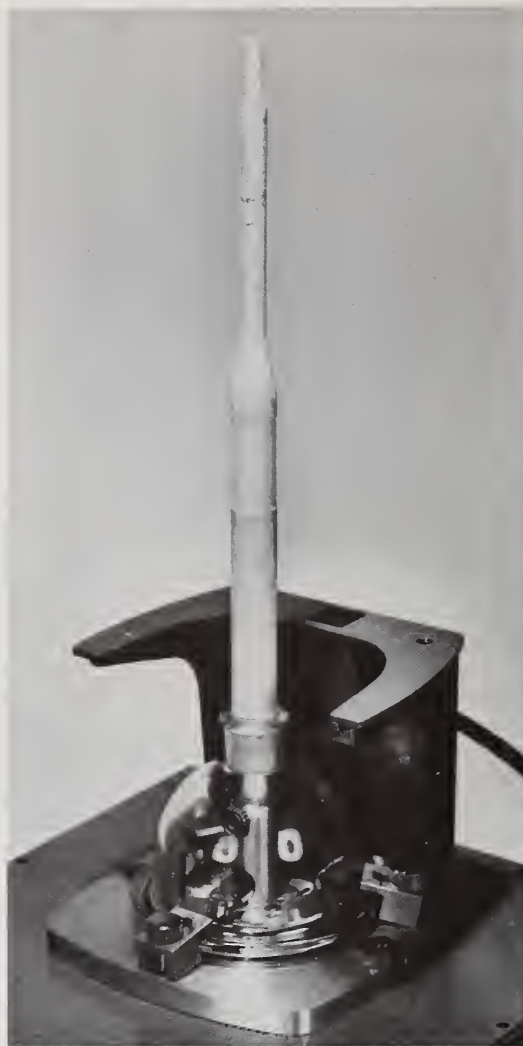
Figure 2. Ceramic tube modification used in research-designed DTA-EGA unit.
