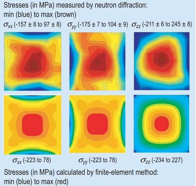
**Fig. 3. Comparison of measured to calculated residual stresses.**  $\sigma_{ij} > 0$  is tensile;  $\sigma_{ij} < 0$  is compressive. The upper panels represent the measurements while the lower panels show the comparable computed stresses.
