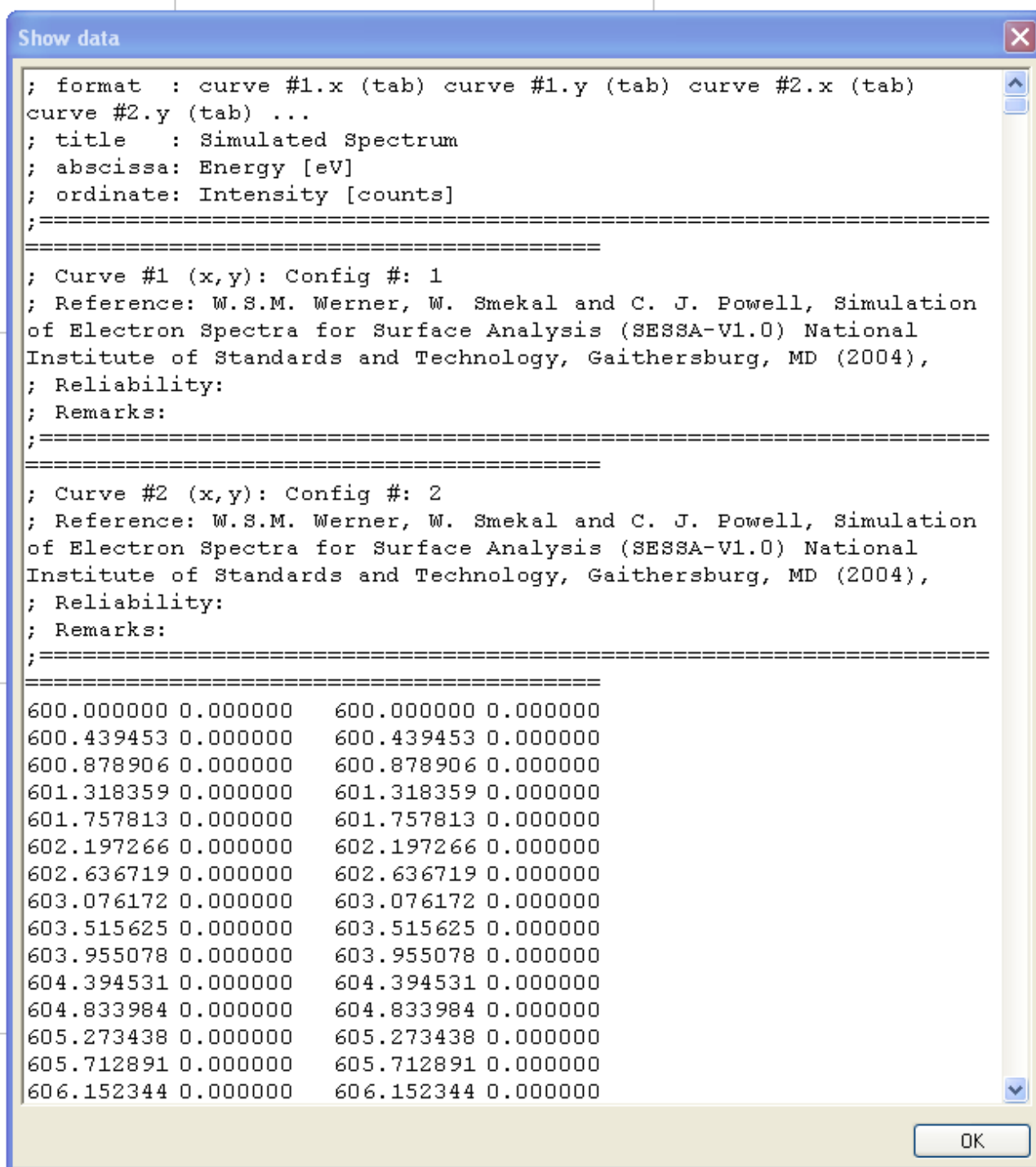
Figure 4.3: Read-only window displaying the data contained in the plot window. The data in this window can be transferred to other software by means of copy and paste operations for further processing.
