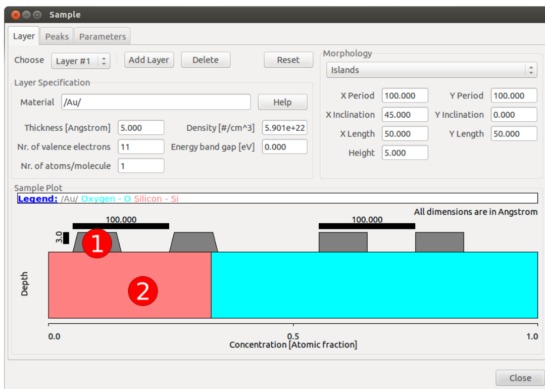
Figure 4.7: Graphical user interface for the SAMPLE Menu for morphology type “islands”. The white numbers in red circles designate layer numbers.
