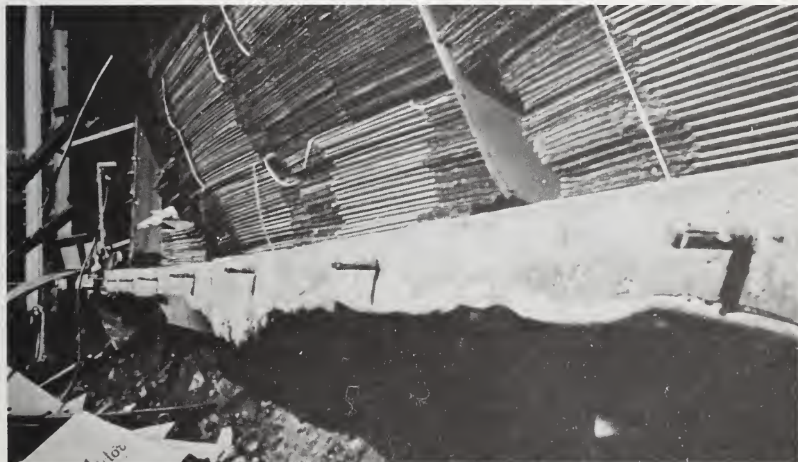
Figure 5.183 Typical failure of drilled-in anchors.
