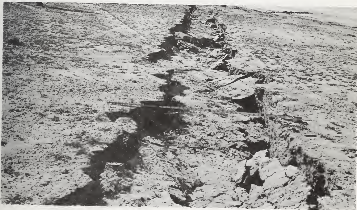
Figure 7.38 Ground cave-in (2-ft wide) near the damaged road slabs shown in figure 7.35.
