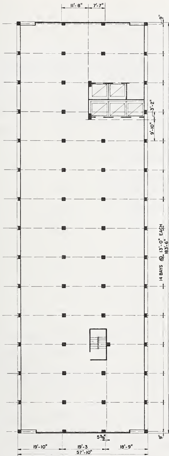
Figure 5.125 Typical floor plan of high-rise section.
