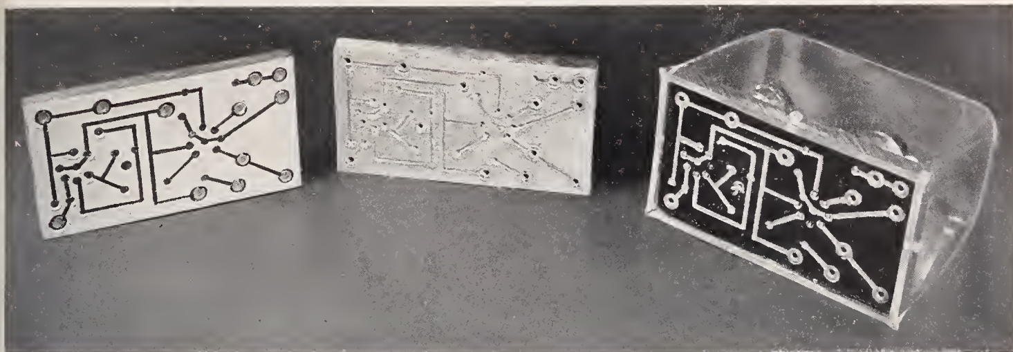
FIGURE 11.1. Three steps in the production of a SPRAYWIRE circuit.
