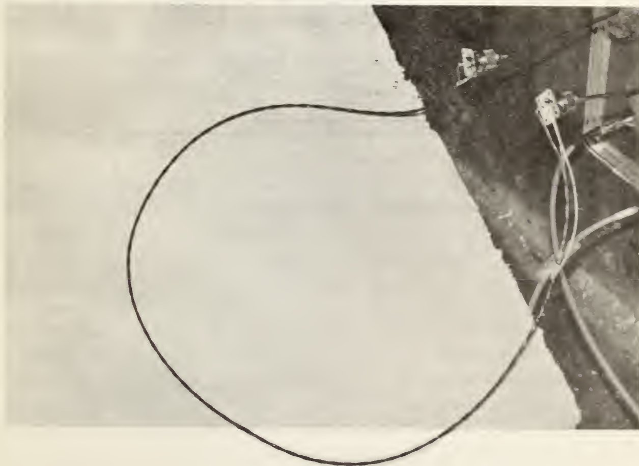
Figure 6. DUT connected to semi-rigid cables inside the chamber.
