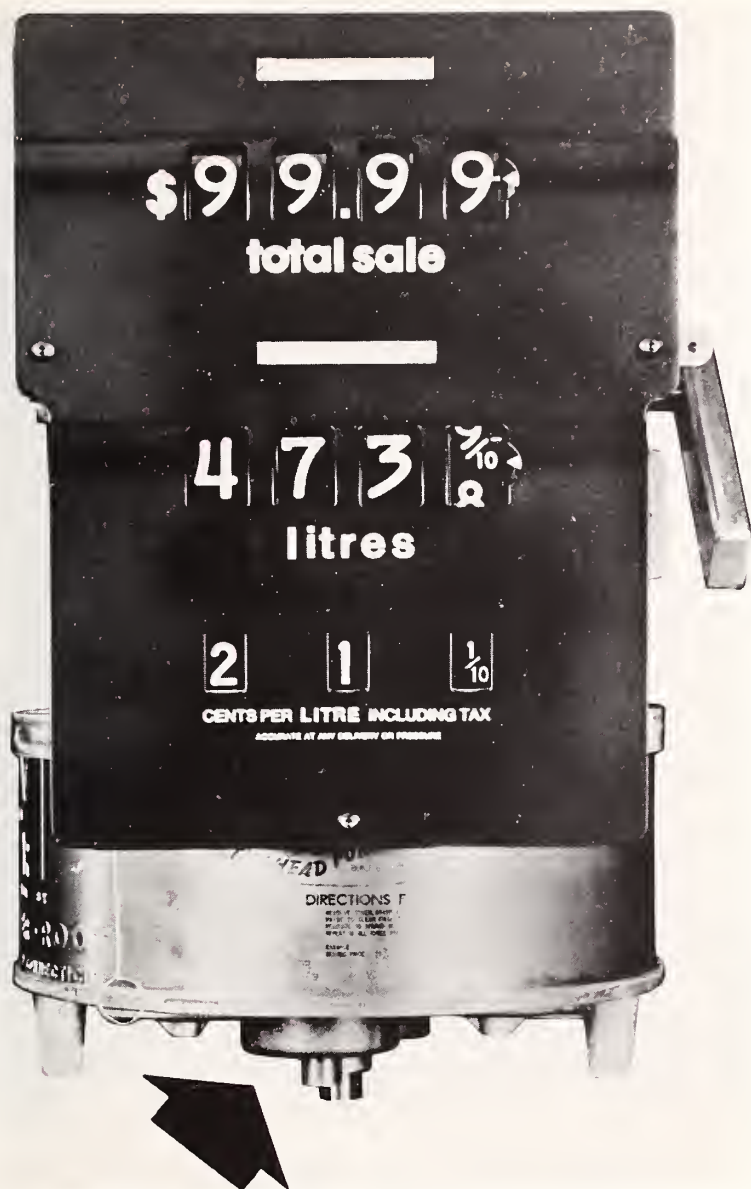
FIGURE 7. 4 Wheel Computer With the Quick-Change Gear Box in the Litre Mode.
