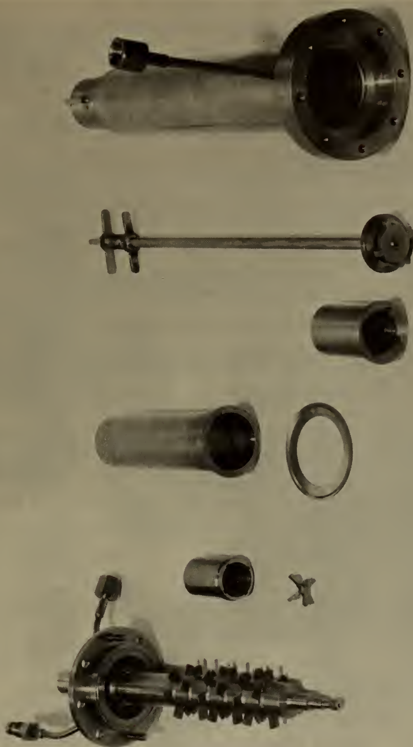
Figure 24. Disassembled cell for use at 1000°C for phase purification
