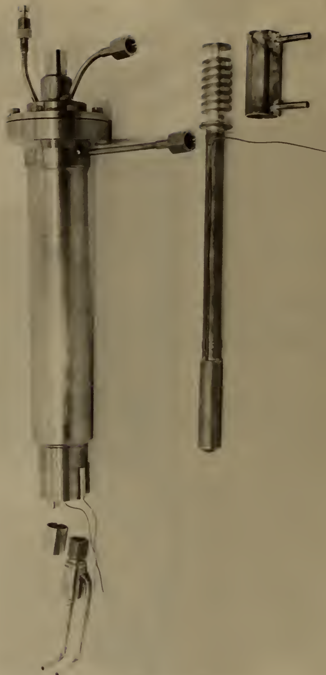
Figure 23. Assembled cell for use at 1000^{\circ}\text{C} in phase purification.
