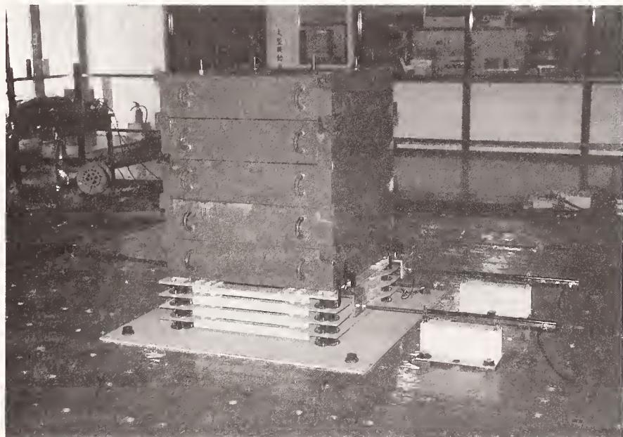
6. **BASIC STRUCTURE (MATERIAL, SHAPE, ETC.)** Material: High damping laminated rubber is arranged in several layers and used as support.
