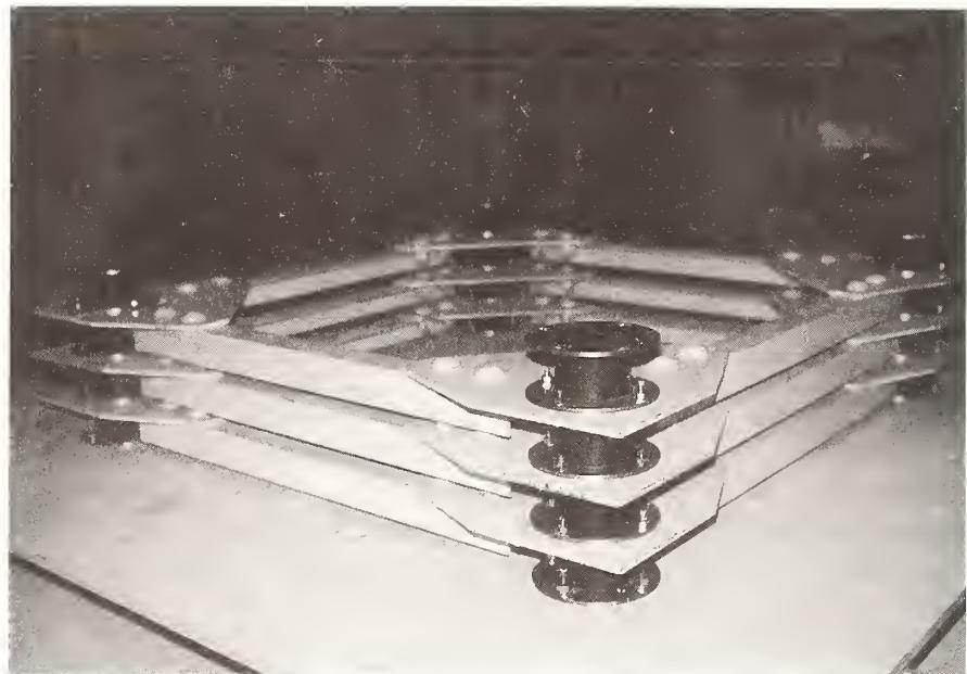
7. **TESTS FOR PERFORMANCE EVALUATION** Excitation test on shaking table
