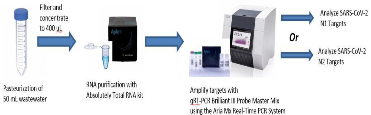
Overview of Weck Laboratories’ workflow for extracting and detecting SARS-CoV-2 RNA in wastewater
