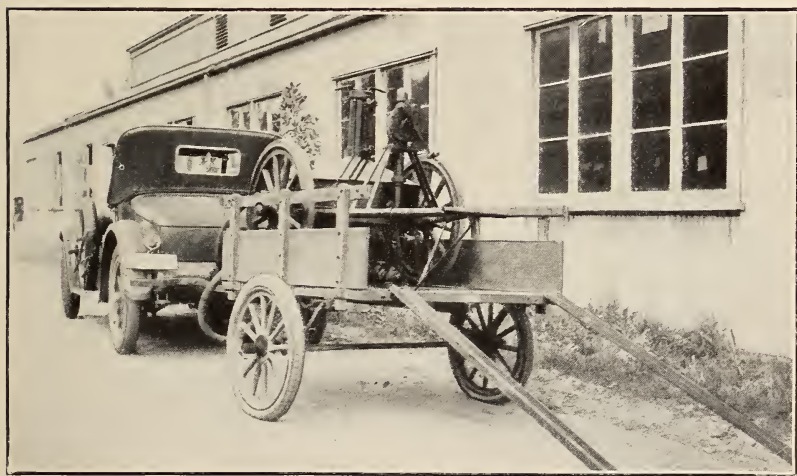
FIG. 7.— Trailer for transporting special 50-gallon measure
