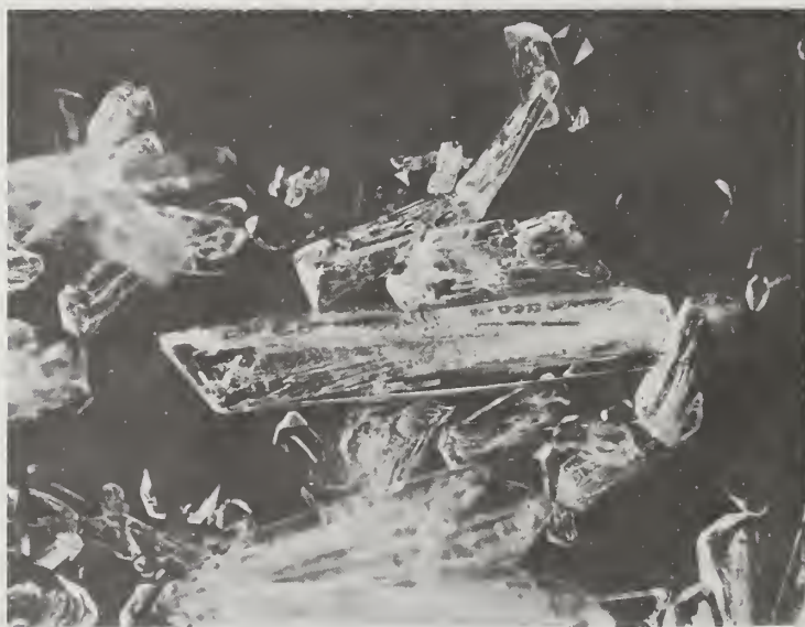
Figure 5. Calcium tartrate crystals grown from aqueous solution in space.
