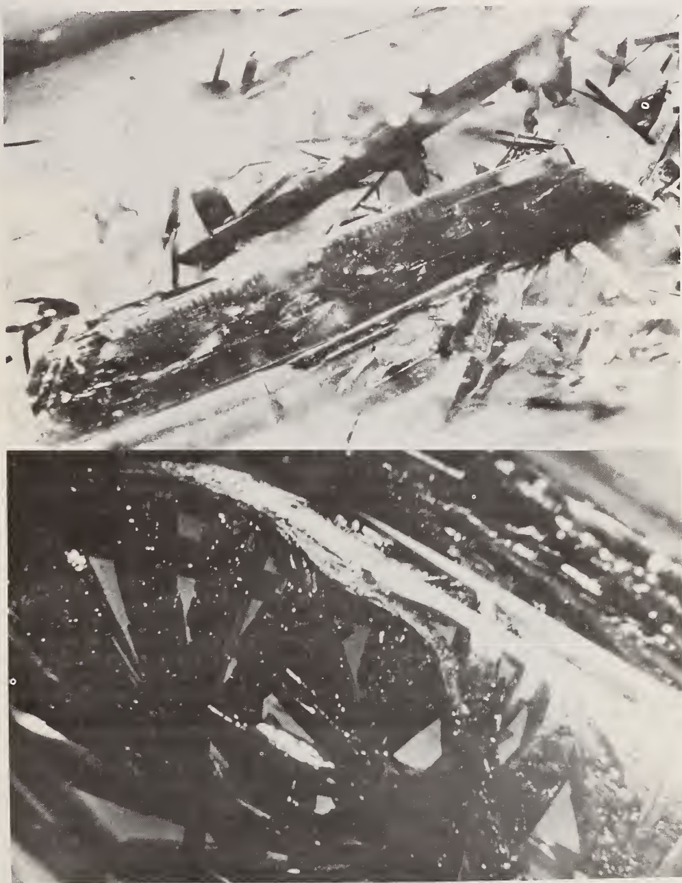
Figure 11. Condensation region of a GeSe transport ampoule. Bottom: Dendritic growth observed on earth. Top: Well developed single crystal platelets grown in space.
