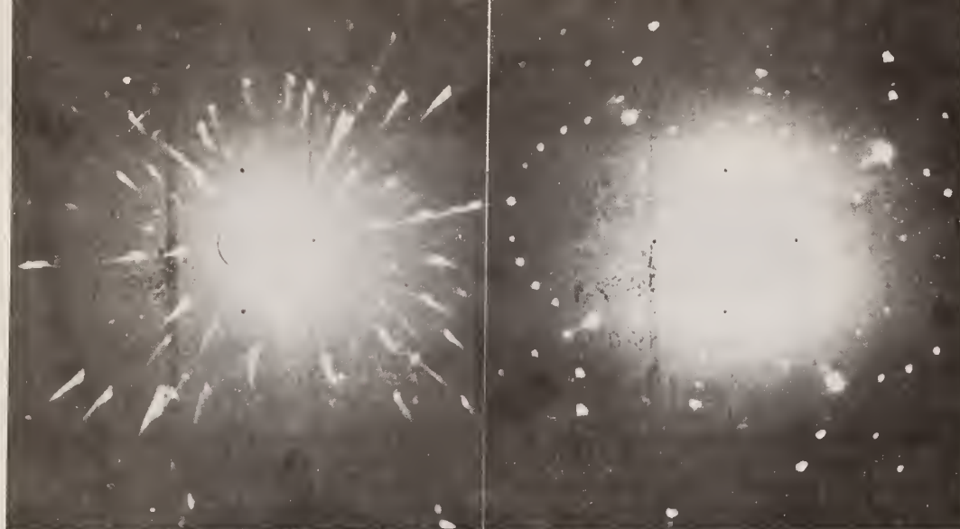
Figure 13. Laue x-ray diffraction transmission photographs of (001) oriented GeSe-GeTe solid solution single crystal platelets. Left: Crystal grown on earth. Right: Crystal grow in space.
