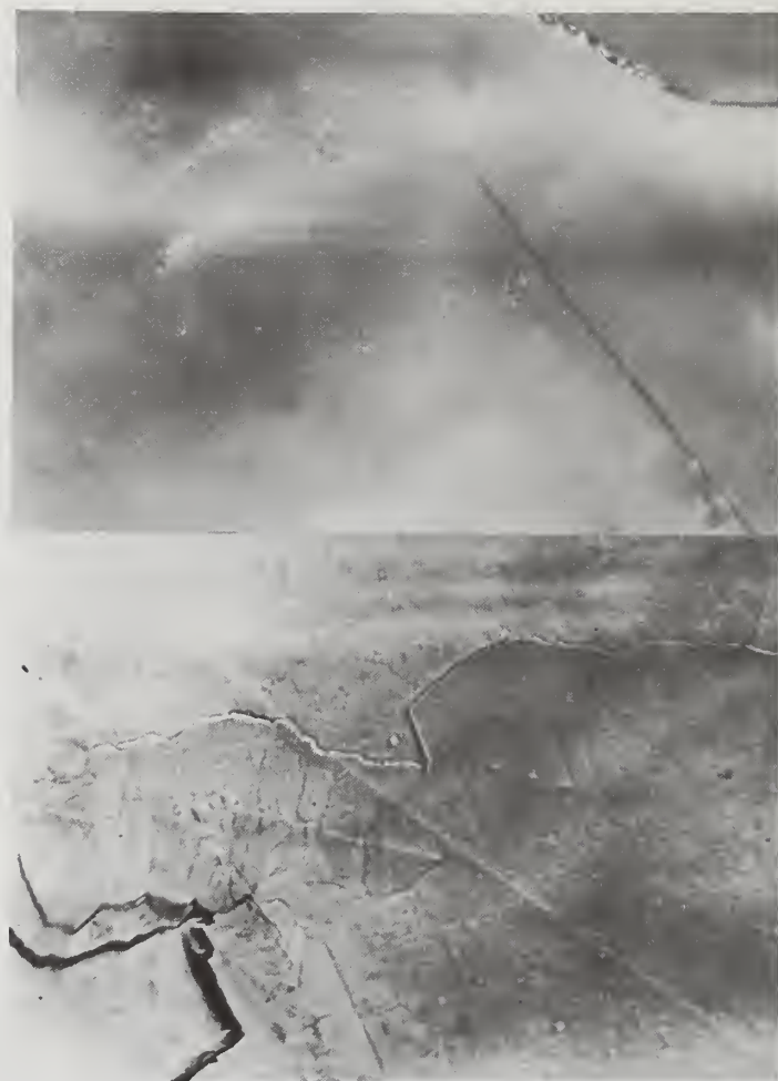
Figure 12. Optical photomicrographs (125 X) of thermally etched cleaved (001) faces of GeSe crystals. Bottom: Crystal grown on earth. Top: Crystal grown in space.
