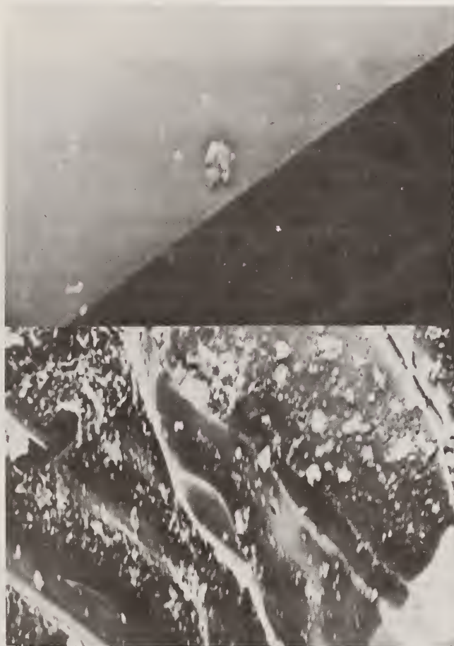
Figure 14. Scanning electron photomicrographs of native faces of GeS-GeSe solid solution single crystals. Top: Crystal grown in space. Bottom: Crystal grown on earth.
