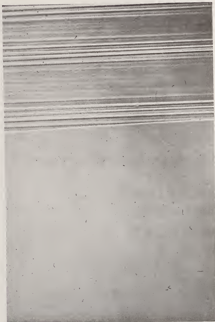
Figure 8. Te segregation behavior revealed by etching in InSb. Top portion: Seed crystal grown on earth. Bottom portion; Regrowth in space.
