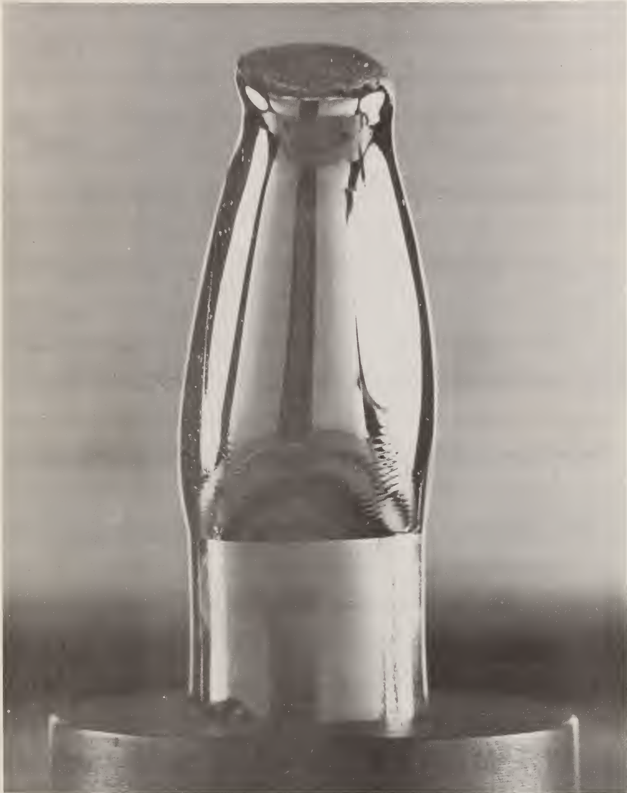
Figure 2. InSb crystal grown by a containerless method in space. Czochralski-grown seed mounted in graphite support at bottom. Boundary between seed and space-grown crystal (top portion) is clearly visible.
