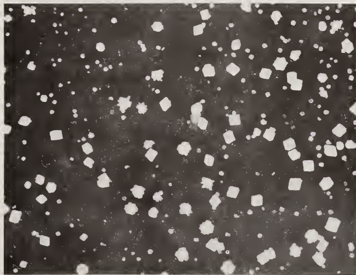
Figure 6. Calcium carbonate crystals grown from aqueous solution in space.
