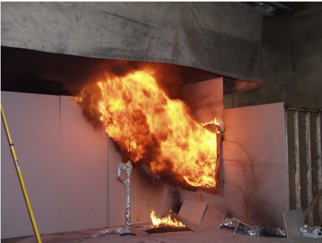
Figure 25 – Exterior View of Window After the Start of Forced Ventilation (380 s)
