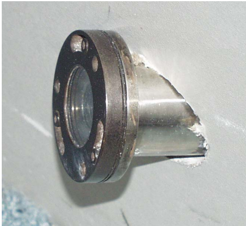
Figure 11 - Water Cooled Camera
