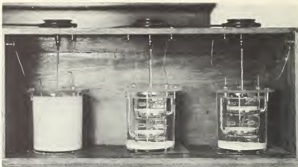
FIGURE 11. Views of the electrolytic preparation of mercurous sulfate. Left vessel—stirrer in operation, cloudiness due to mercurous sulfate suspended in solution. Center and right vessels—stirring stopped, mercurous sulfate at bottom of vessels and on surface of mercury in dishes.
