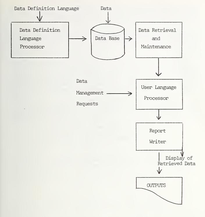
FIGURE 2. DBMS Functional Components.
