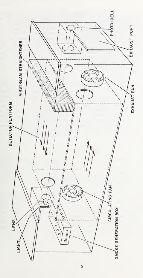
SMOKE DETECTOR TEST CHAMBER
