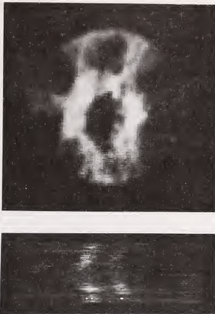
Figure 11 The top image shows a two-dimensional reconstruction of the variance in refractive index (temperature dependent) from eleven experiments. The image on the bottom is the profile data used to make the reconstruction at the top. The profile data shown represents the variance of eleven profiles, each corresponding to one of eleven experiments. See Figure 7 for data format.
