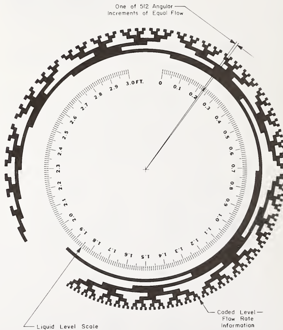
Figure 8 - Opto-Electronic Function Generator Level-to-Flow Rate Conversion System.
