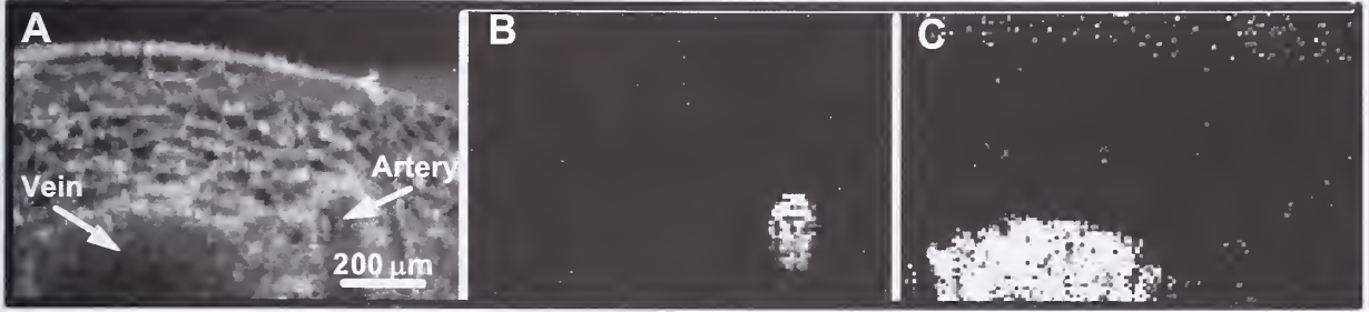
Figure 1: Doppler OCT images of in vivo rodent mesentery blood flow. OCT structural image (A), with white and black representing high (80 dB) and low (0 dB) backscattered light intensities, respectively. ODT velocity image of blood flow in artery (B), white and black represent high (4000 \mu\text{m/s} ) and zero velocity, respectively. Velocity image of blood flow in veins (C), white and black represent high (1000 \mu\text{m/s} ) and zero velocity, respectively.
