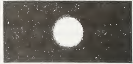
Fig. 3. Typical visible output far-field pattern from one of the tapered fibres.
