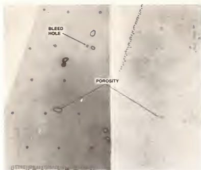
Figure 8. Chem-milled portion of DATUS 8 with recording.
