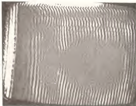
Figure 4. Acoustic micrograph of portion of flawed CDR06 BX chip. Gross delamination is indicated by opaque areas. 30X magnification.
