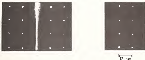
Figure 9. Fourier plane from figure 7 after correcting the distortion and image of wire array after correcting the distortion.
