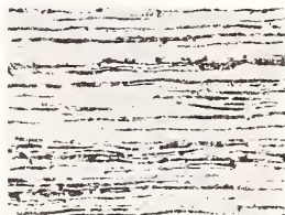
Figure 3b. Pearlite banding in alloy C after annealing at 1650 °F (50 X, Nital etch).
