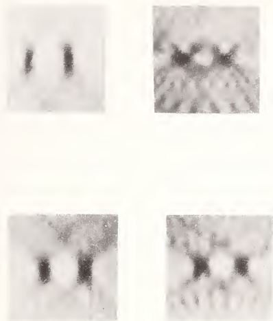
Figure 7. Reconstruction with 31 rays and field of view of (a) 75°, (b) 100°, (c) 125°, and (d) 150°.
