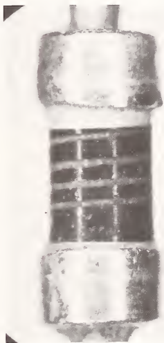
Figure 7. Unencapsulated tin-oxide resistor showing spiral trimming grooves. 30X magnification.
