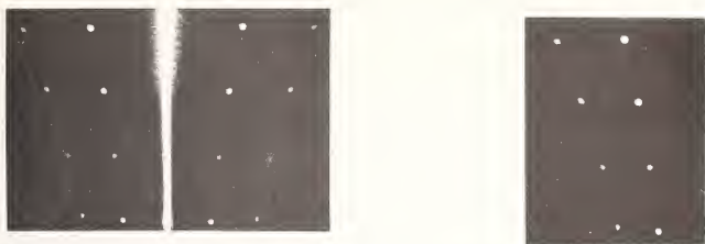
Figure 8. Fourier plane from figure 7 showing isoclinic distortion and image of wire array showing isoclinic distortion.
