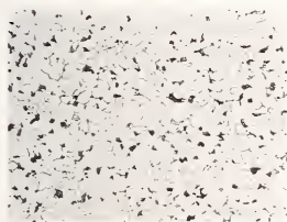
Figure 3a. Polygonal ferrite and pearlite in alloy G after annealing at 1600 °F (100X, Nital etch).
