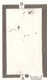
Figure 3. (a) Acoustic amplitude image of a typical moly preform. (b) Acoustic phase variation (upper curve) and acoustic amplitude variation (lower curve) along line A-B of (a).
