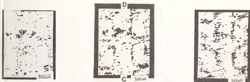
Figure 4. Acoustic amplitude images of a portion of the power transistor obtained with different adjustment of focus. (a) focused on the silicon surface, (b) focused at the silicon-alloy interface, and (c) focused on the transistor back surface.
