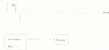
Figure 1(a). The electronic box allows digital control of frequency, burst number and recurrence period over wide ranges. It includes a transmit/receive switch, power amplifier, and other sonar type circuits.
