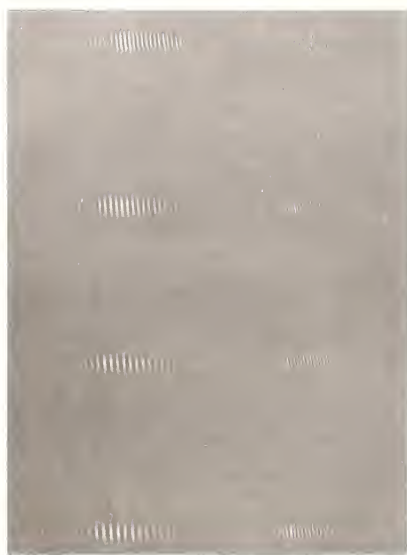
Figure 7. Hologram formed by scanning the array of wires of figure 6.
