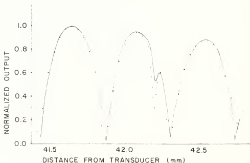
Figure 5. Optical scan of compressional wave in 7070 pyrex with bubble defect. Experimental data is indicated by solid circles; data calculated assuming circular bubble and Gaussian optical beam profiles by solid line.
