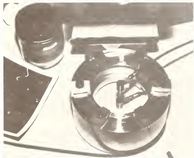
Figure 1. Apparatus for the investigation of ultrasonic interactions with thin air layers between fused silica optical flats.
