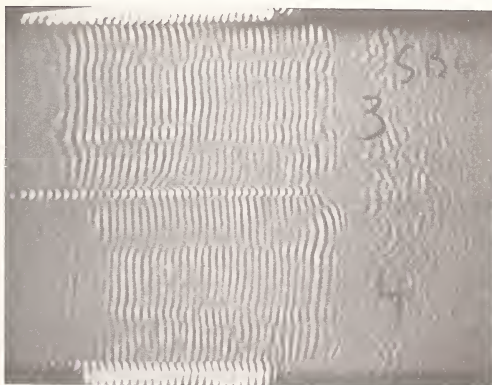
Figure 2. - Acoustic micrograph of two CDR02 BX chip capacitors. Top chip shows misalignment in electrode stack; bottom chip shows well-centered electrode stacking. 30X magnification.
