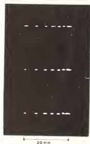
Figure 11. Image of wire array in figure 10. Isoclinic distortion corrected.
