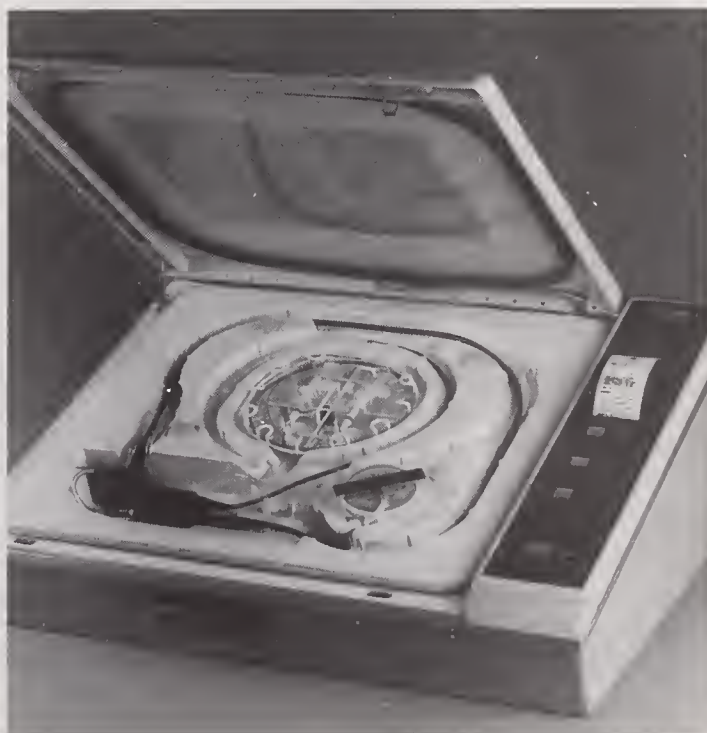
Figure 8. STERIS SYSTEM 1™ sterilization unit showing the complex shape of the instrument tray necessary for sterilization of an endoscope.
