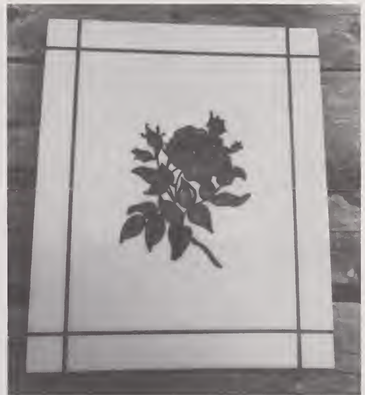
Figure 1. Rose inlay created by routing out a pattern in the acrylic countertop material and then filling with material that is usually used to make repairs in the countertop materials. This illustrates the versatility of the computer-controlled router for making complex shapes.
