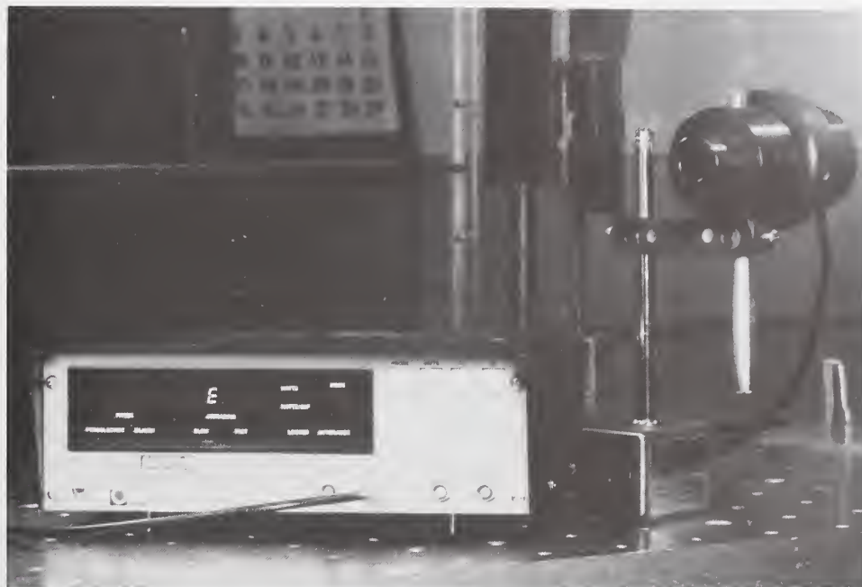
Commercial, electrically calibrated optical power meter based on NBS design.
