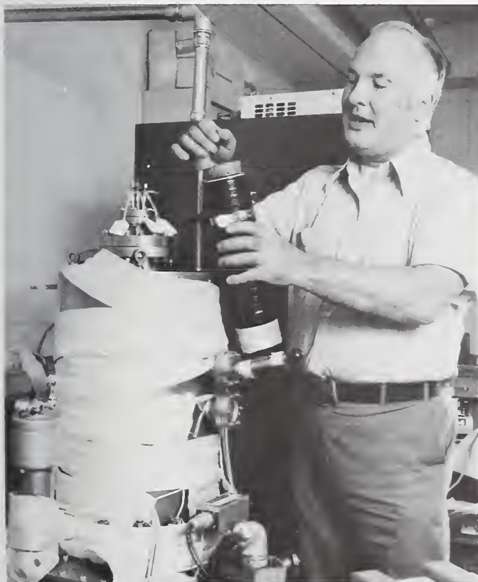
George Burns, making reference junction connections in an ice bath, in preparation for thermocouple calibration.
