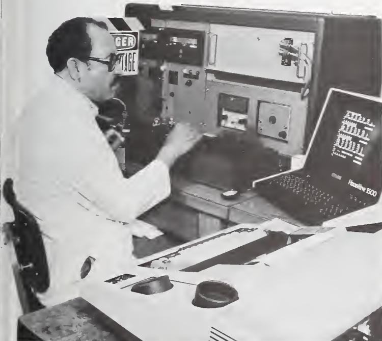
Cliff Childers, carrying out AC-DC difference calibrations.
