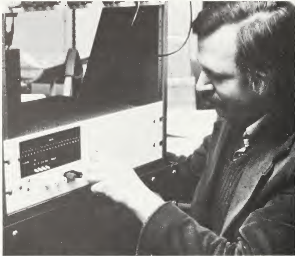
Michael Souders, working on development of NBS system for characterizing analog-to-digital and digital-to-analog data converters.
