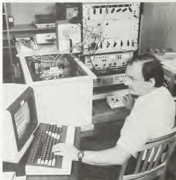
Charles Levy, conducting electrical conductivity measurements of non-ferrous standards.
