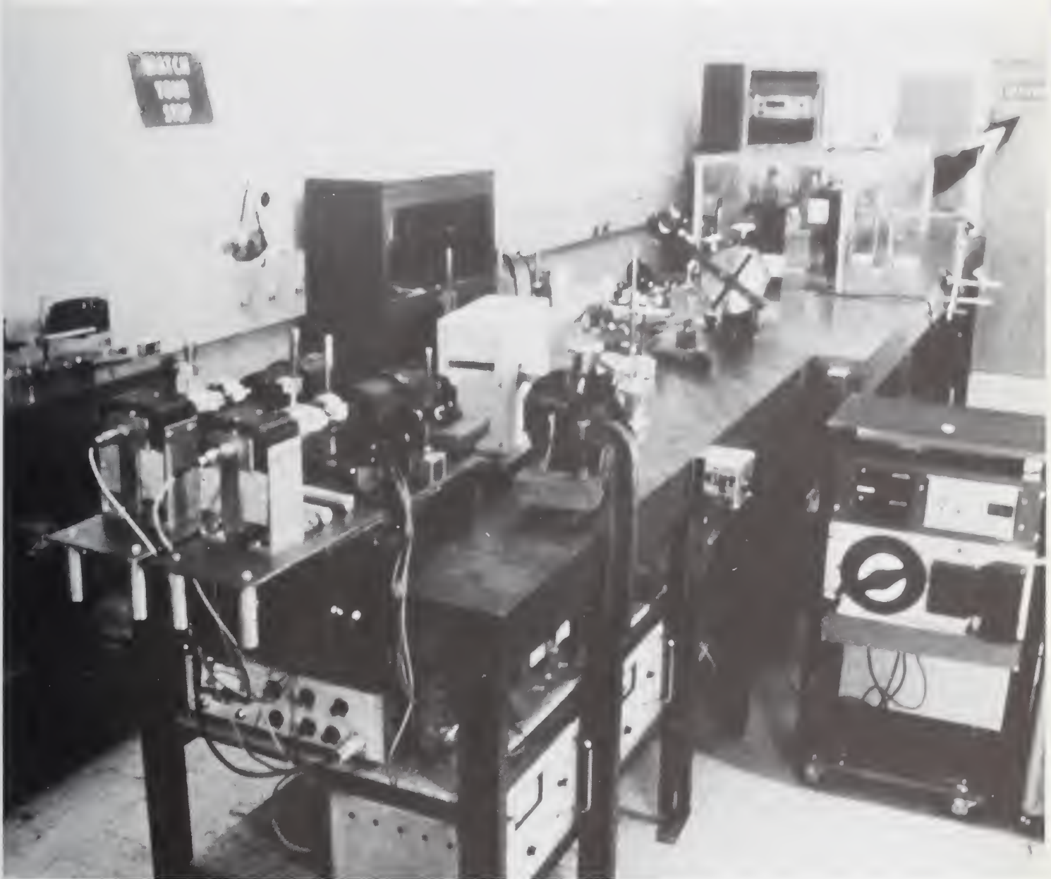
Apparatus for comparing customer's laser power meter (calorimeter) with NBS reference calorimeter.
