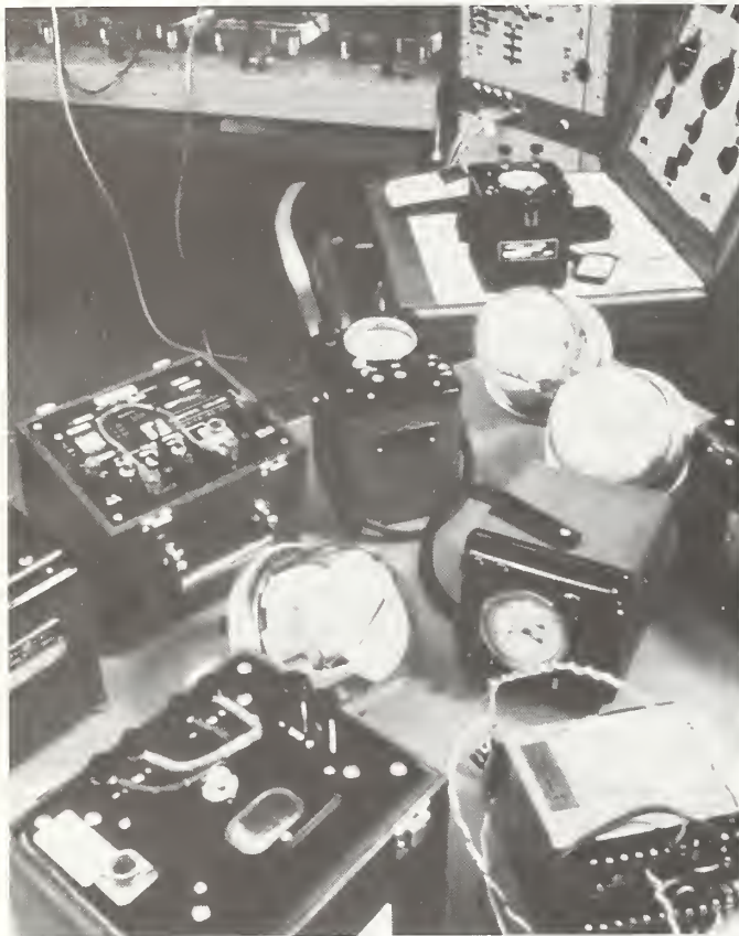
Foreground: NBS reference wattmeters, watthour meters. Background: NBS electrical power and energy measurement system.
