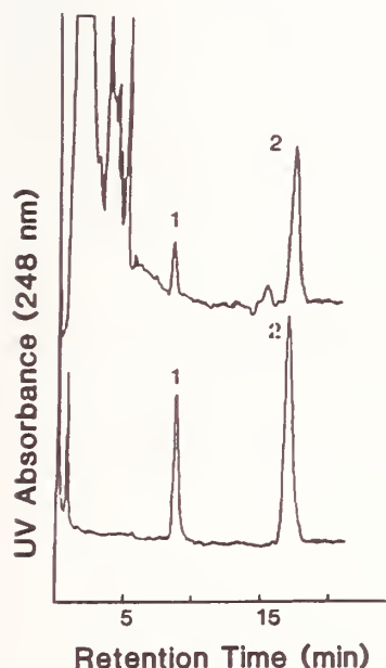
Fig. 2. Lower trace: HPLC from the analysis of a standard solution of (1) 1 \mu\text{g/ml} GRA and (2) 3.4 \mu\text{g/ml} GRA acetate using methanol–water–acetic acid (75:24.7:0.3, v/v) at a flow-rate of 2 ml/min on a C_{18} column with UV detection at 248 nm. Responses shown represent 30 ng GRA and 90 ng GRA acetate. Upper trace: HPLC from the analysis of plasma extract using solid-phase extraction: (1) 0.38 \mu\text{g/ml} GRA and (2) 2.9 \mu\text{g/ml} GRA acetate.
