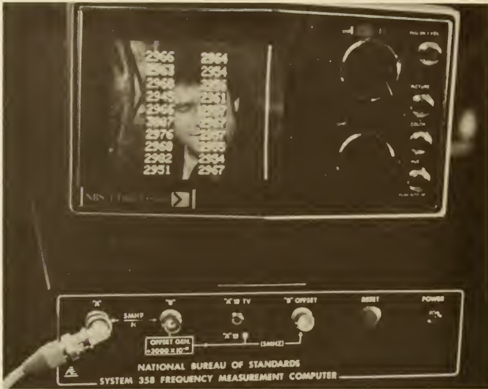
FIGURE 7.5. THE NBS PROTOTYPE, SYSTEM 358 FREQUENCY MEASUREMENT COMPUTER.
