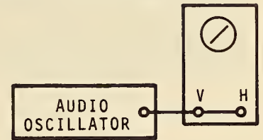
FIGURE 4.26. EQUIPMENT HOOKUP FOR A 1:1 LISSAJOUS PATTERN.
