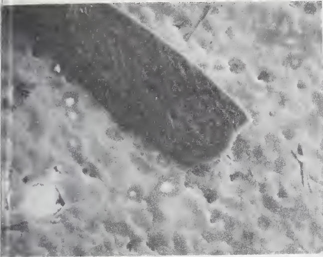
Figure 15. Scanning electron micrograph of the surface of the thick-film gold metallization used in these ultrasonic bonding experiments. (Magnification: \sim 400\times .)
