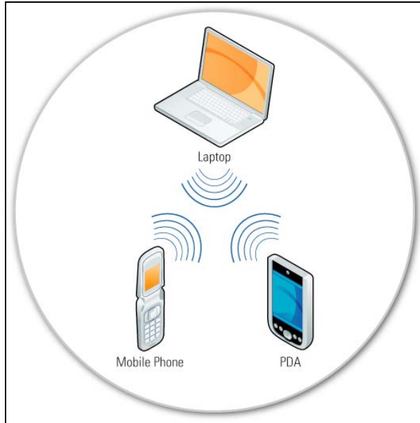
Figure 2-1. IEEE 802.11 Ad Hoc Mode Architecture
