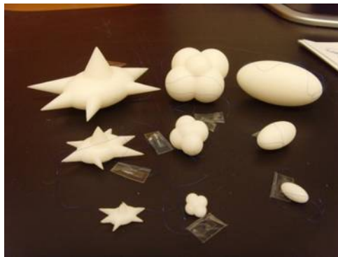
Figure 1. Figure showing FDA non-spherical phantom nodules (courtesy of Marios Gavrielides, Center for Devices & Radiological Health, US Food & Drug Administration).
